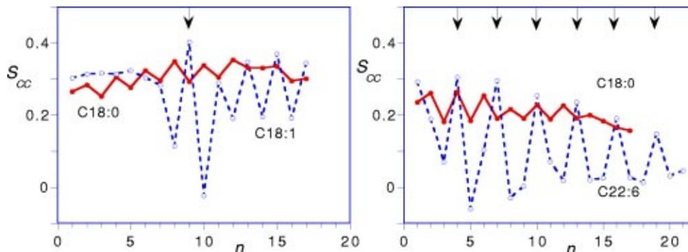
FIG. 7. Order parameter  $S_{CC}$  as a function of the bond number  $n$  of the lipid hydrocarbon chains of the bilayers as determined from the MD simulations. The arrows indicate the double bonds.
