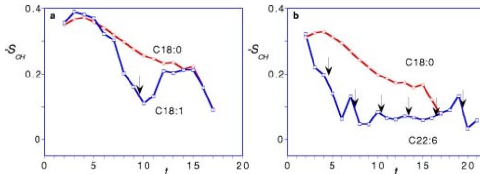
FIG. 4. Order-parameter profiles  $-S_{CH}$  for both tails of the lipid molecules of SOPC and SDPC as determined from the SCF calculations;  $t$  is the segment number along the chain. The arrows indicate the positions of double bonds.
