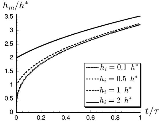
FIG. 4. Short-time evolution of the rim height  $h_m$ , plot of  $h_m$  versus  $t/\tau$ , for  $h_i = 0.1, 0.5, 1$ , and  $2h^*$ . Note that the curves corresponding to  $h_i = 0.1$  and  $0.5h^*$  cannot be distinguished within the graph scale.
