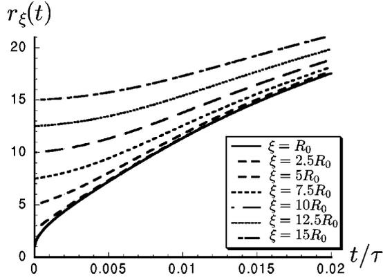
FIG. 13. Graphic representation of characteristics  $r_\xi(t)$ , for an initial thickness  $h_i = 0.1h^*$  and  $t$  ranging from 0 to  $0.02\tau$ . Different values of  $\xi$  parameter are taken as  $\xi = 1, 2.5, 5, 7.5, 10, 12.5$ , and  $15R_0$ .
