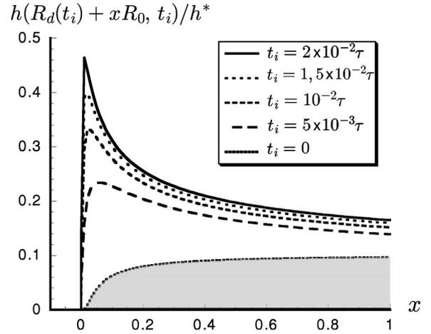
FIG. 14. Evolution of the film morphology near the hole periphery (from  $R_d$  to  $R_d + R_0$ ), starting with a continuous profile [Eq. (E2) with  $\chi = 0.1$ , filled with gray color]. Each profile, which is relative to the time  $t_i$  and describes the domain  $r \geq R_d(t_i)$ , is shifted to the point  $x = [r - R_d(t_i)] / R_0 = 0$ , so as to exhibit clearly its increasingly asymmetric shape.
