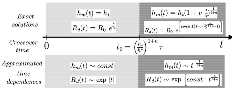
FIG. 12. Summary of the different time regimes for the dewetting of thick films ( $h_i \gg h^*$ ). Depending on each time range, the exact solutions and corresponding approximated time dependences are precised.
