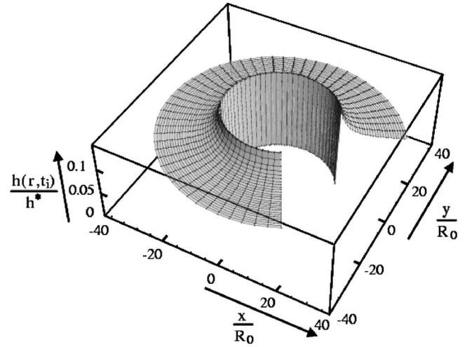
FIG. 7. Film profile for  $h_i = 0.1h^*$  and  $t = 2 \times 10^{-2}\tau$ . The constitutive equation of the material is the Cross law [Eq. (4)], with a power-law index  $n = 2/3$ . For clarity reasons, a sectional view is displayed on a quarter of a circle, and Cartesian coordinates  $(x, y, z)$ , naturally associated with cylindrical ones  $(r, \Phi, z)$ , are used.
