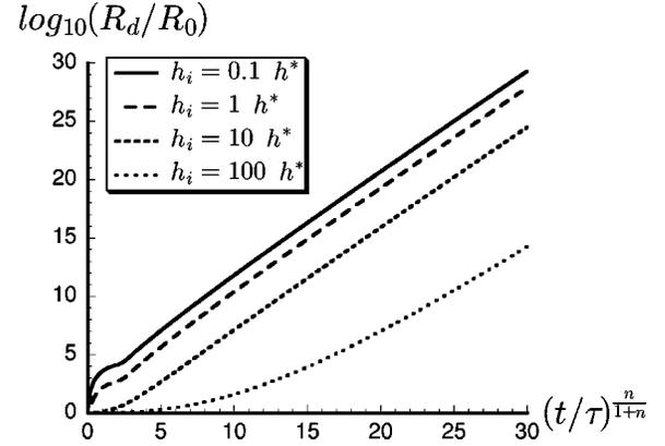
FIG. 9. Logarithmic plot of the dry zone radius  $R_d$  versus  $(t/\tau)^{n/(1+n)}$ , for  $h_i = 0.1, 1, 10,$  and  $100h^*$ , in the case of Cross law with  $n = 2/3$  and  $k = 5$ . Note the linear behavior of  $\log_{10}[R_d(t)/R_0]$  with  $(t/\tau)^{n/(1+n)}$  after a transient time: the anticipated stretched exponential [Eq. (24)] is indeed obeyed.
