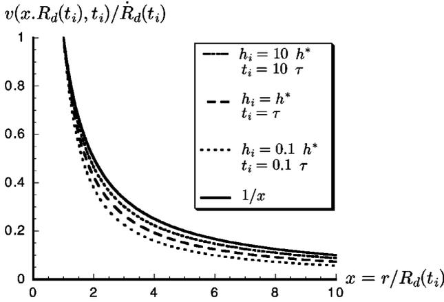
FIG. 10. Velocity field  $v(r, t_i)$  for different initial thicknesses ( $h_i = 0.1, 1, 10h^*$ ), at a given time  $t_i$ . All radial distances are normalized by the dry radius at time  $t_i$  for each thickness. A curve  $1/x$  is represented for comparison. It is clear that the velocity field is almost proportional to  $1/r$  for a thick profile ( $h_i = 10h^*$ ), similar to the long range radial plug flow observed by Debrégeas.
