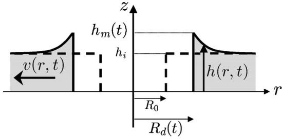
FIG. 1. Film geometry:  $h(r,t)$  is the profile of the film,  $h_m(t)$  is the height of the rim, and  $R_d(t)$  is the radius of the dry zone. The initial ( $t=0$ ) steplike profile is represented by the dashed line.  $v(r,t)$  is the radial, axisymmetric flow field.
