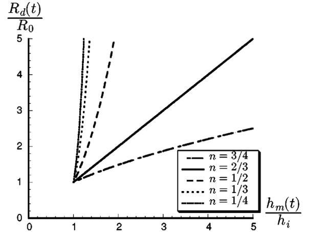
FIG. 5. For thin films ( $h_i \ll h^*$ ), during the initial stages of the growth, the dry radius is related to the rim height by a simple power law depending on the material rheology [Eq. (19)]. This figure shows the different regimes depending on  $n$ : for  $n = 2/3$ , the dependence is simply linear; for  $n > 2/3$ , the radius grows slower than the rim height, while for  $n < 2/3$ ,  $R_d$  grows fastly compared to the rim height increasing.
