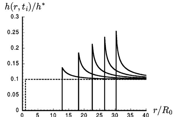
FIG. 8. Evolution of a film (Cross model,  $n = 2/3$ ) profile  $h(r, t_i)$ , for  $h_i = 0.1h^*$  and  $t_i$  ranging from  $t = 0$  (initial configuration, in dashed lines) to  $t = 5 \times 10^{-2}\tau$  with a time step of  $10^{-2}\tau$ .
