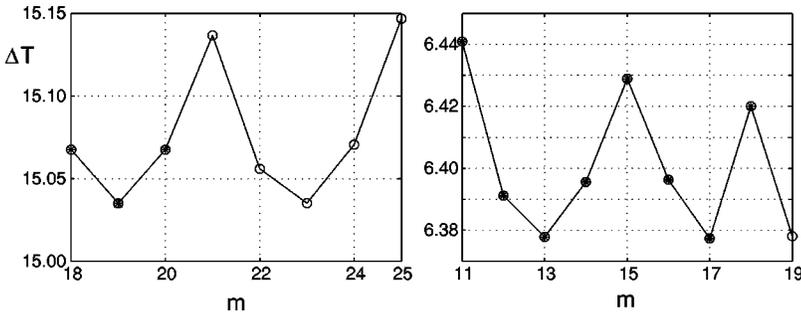
FIG. 4. Marginal stability diagrams which show  $\Delta T_c$  vs the wave number  $m$  at different physical conditions. Filled black circles indicate complex eigenvalue while nonfilled circles correspond to a real eigenvalue. (a) A codimension two bifurcation of stationary and oscillatory modes at  $\Delta T_h = 6$  °C,  $B = 0.25$  and  $\Delta T_c = 15.04$  °C. (b) Competition of one stationary and two oscillatory modes at  $\Delta T_h = 5$  °C,  $B = 0.85$ , and  $\Delta T_c = 6.36$  °C.
