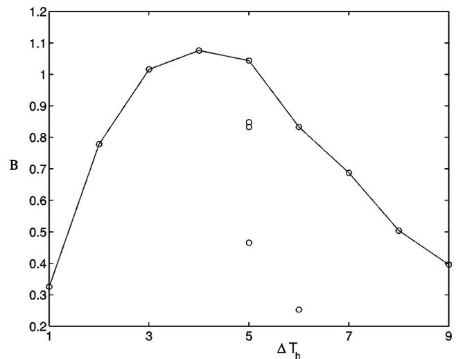
FIG. 5. Biot number at which a codimension-two bifurcation point appears for different  $\Delta T_h$  values.
