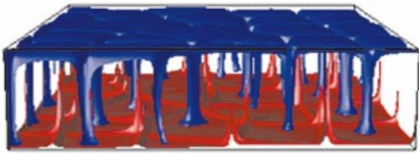
FIG. 2. (Color) Hot and cold isotherm surfaces from RBI simulation of Ref. [19], R \approx 10^6 .
