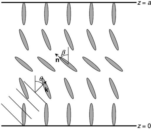
FIG. 1. Geometry of a sound wave interacting with a liquid crystal in a cell of thickness  $a$ . The homeotropic boundary conditions fix the director at the two surfaces of the cell, so the molecules can only realign in the interior of the cell.
