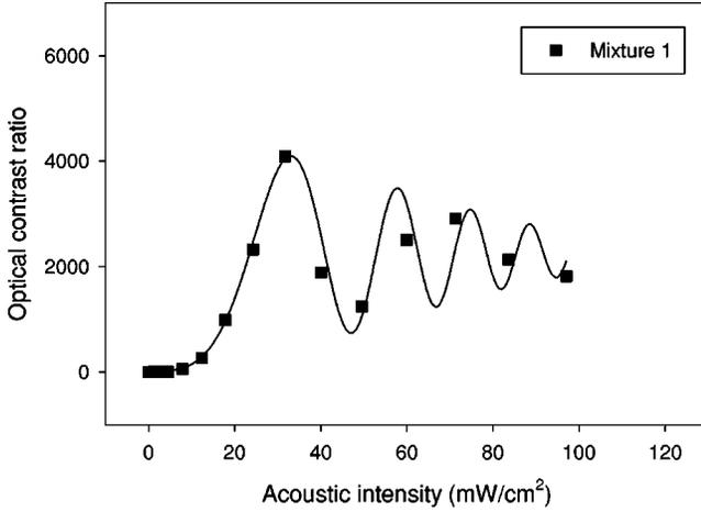
FIG. 4. The modified fit for the optical contrast ratio of mixture 1, using the Gaussian distribution of acoustic intensity discussed in the text. The oscillations in the contrast ratio beyond the first peak are damped out.
