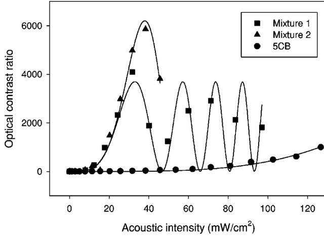
FIG. 3. Symbols: Data for optical contrast ratio as a function of acoustic intensity for the three liquid crystal samples. Mixture 1 is measured at the peak angle of  $\theta_{\text{water}} = -8^\circ$ , mixture 2 at  $+8^\circ$ , and 5CB at  $-5.5^\circ$ . Lines: Fits of the data to the prediction of Eq. (15).
