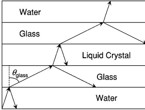
FIG. 2. A sound wave travels through a multilayer environment of water / glass / liquid crystal / glass / water, with partial transmission and partial reflection at each interface (not to scale).
