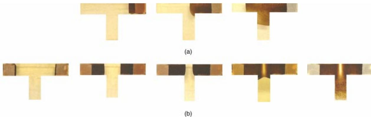
FIG. 2. Photographs of experimental implementation of the XOR gate. (a) The progression of the reaction-diffusion gate for the inputs  $x=F$  and  $y=T$ . (b) The progression of the reaction-diffusion gate for the inputs  $x=T$  and  $y=T$ .
