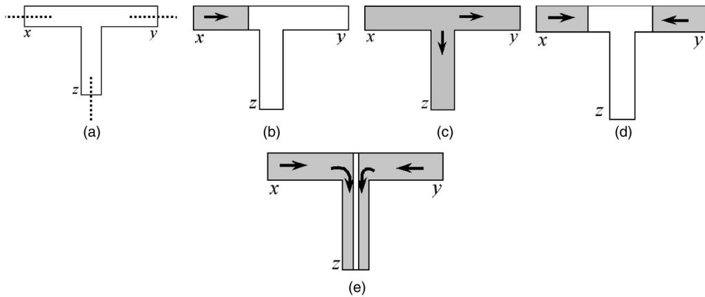
FIG. 1. Schematic action of the XOR gate. (a) An architecture of the gate; sites where state of the reactor is measured are shown by dotted lines. (b) One of the inputs gets a reactant,  $x=T$ , the reactant diffuses along the gate chambers and (c) reaches an output,  $z=T$ . (d) Both outputs get the reactant,  $x=y=T$ , two wave fronts of the reactant move towards one another, they interact and form an uncolored bisector (e),  $z=F$ .
