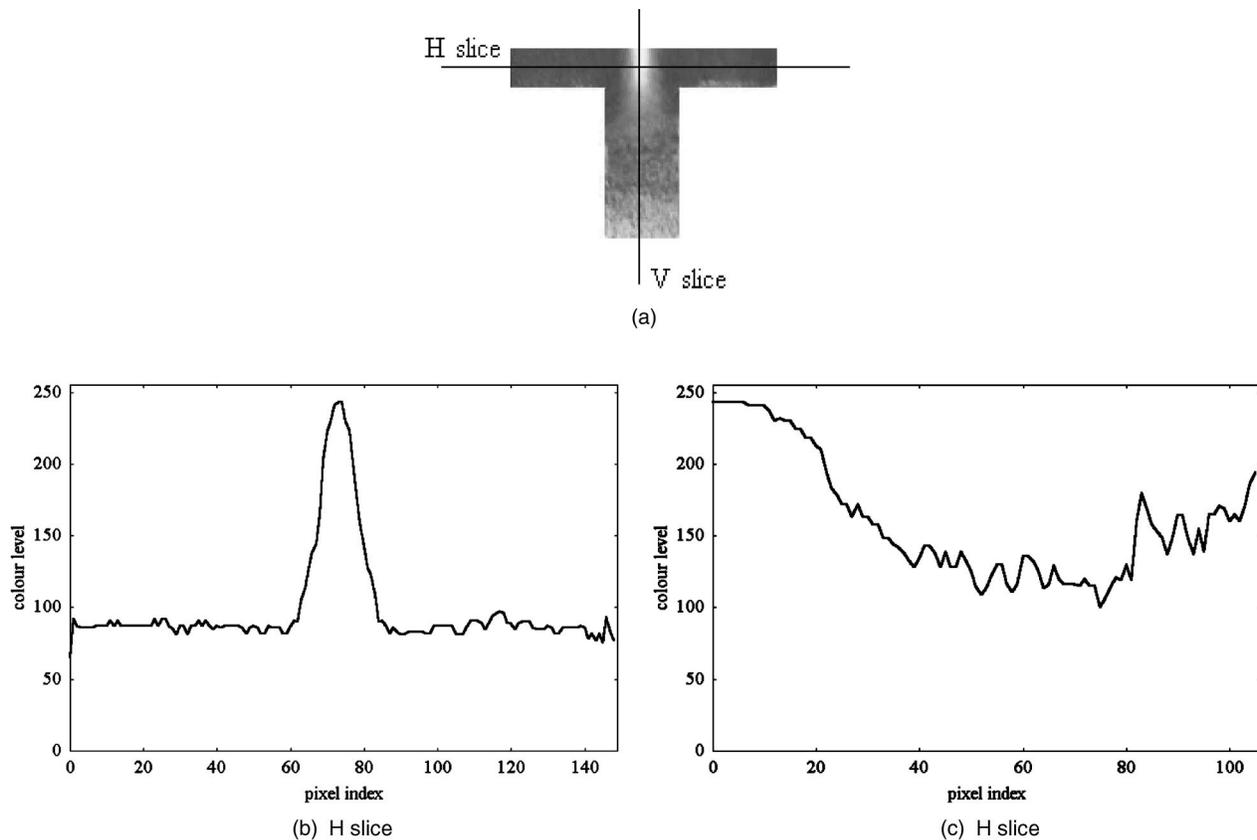
FIG. 3. An example of the value  $T$  representation in concentration of precipitate. The diagram shows a one-pixel horizontal (b) and vertical (c), see scheme (a), slices of the 8-bit-per-pixel image of the experimental realization of the XOR gate [Fig. 2(b), bottom image].
