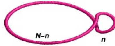
FIG. 2. (Color online only) A closed loop ( N -monomer polymer) folded into a shape that can be approximately described as two circles consisting of N-n and n monomers, separated from each other by a distance of order n monomer sizes.
