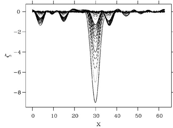
FIG. 4. Evolution according to the generic equation (67).  $\alpha = 0.8$ ,  $\beta = 1.0$ . The initial interface is a random structure (visible near  $z=0$ ). Time interval between curves is  $\Delta t = 1.0$  up to  $t = 20.0$ , thereafter  $\Delta t = 0.1$ , and the evolution is shown up to  $t = 21.6$ . Note the spectacular acceleration of the “winning groove.”
