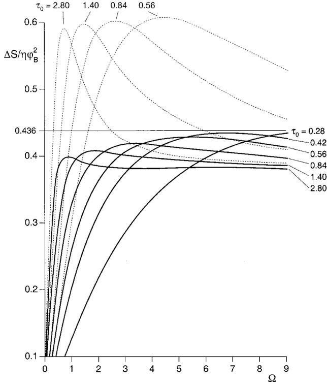
FIG. 5. Comparison of the numerical results of Fig. 3, relative to terminated artificial lines of several lengths (continuous curves), and the results of Fig. 4, relative to open lines (dashed curves). The horizontal line situated at  $0.436\eta\phi_B^2$  corresponds to Eq. (6).
