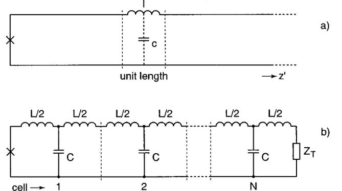
FIG. 1. Josephson junction coupled to an open transmission line (a), where  $l$  and  $c$  represent the inductance and the capacitance per unit length. In (b), the junction is coupled to an artificial line consisting of  $N$  cells of  $T$  type, terminated with the impedance  $Z_T$ .
