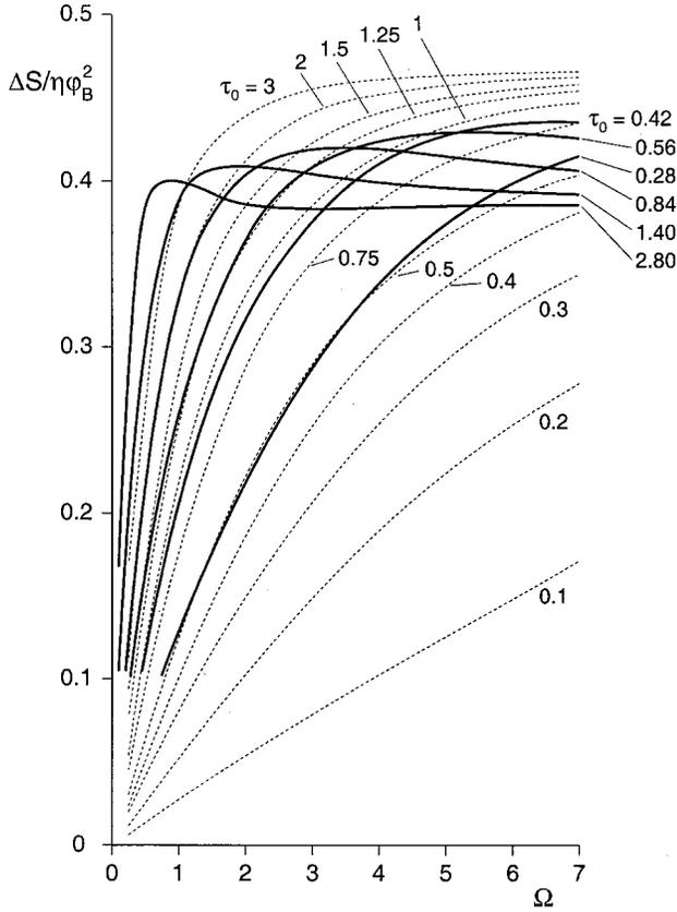
FIG. 3. Increase of the action  $\Delta S$  in units of  $\eta\phi_B^2$  (continuous lines) as a function of the angular frequency  $\Omega$  of the bounce trajectory, computed for different values of the delay  $\tau_0$  of the artificial line consisting of  $N=2-20$  cells, terminated with  $Z_T=Z_0$ . The dashed curves represent the results of the formula in point (f) of Table I, divided by two. The agreement is acceptable only in the large  $\Omega$  limit.
