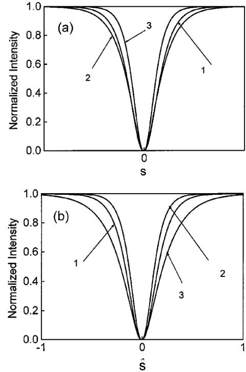
FIG. 3. Dark-dark separate screening soliton pairs in a biased series SBN crystal circuit. (a) Dark soliton profiles in the crystal  $P$ . (b) Dark soliton profiles in the crystal  $\hat{P}$ .
