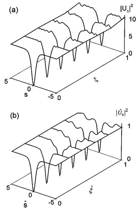
FIG. 7. Dynamical evolutions of the two dark solitary states  $U_1$  and  $\hat{U}_0$  in a biased series SBN crystal circuit. (a)  $U_1$  in the crystal  $P$  and (b)  $\hat{U}_0$  in the crystal  $\hat{P}$ .
