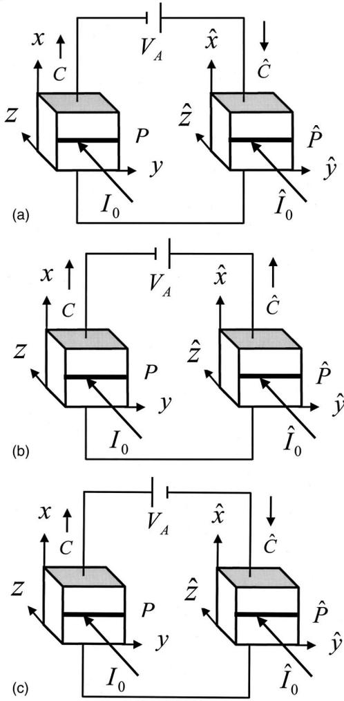
FIG. 1. Illustration of a biased series PR crystal circuit consisting of two PR crystals to support a bright-bright soliton pair in (a), a bright-dark soliton pair in (b), and a dark-dark soliton in (c).  $P$  and  $\hat{P}$  denote the two crystals, respectively.  $C$  and  $\hat{C}$  denote the two  $c$  axes.  $I_0$  and  $\hat{I}_0$  denote the incident bright or dark solitonlike in one-dimensional laser beams.  $V_A$  denotes the voltage of the source.
