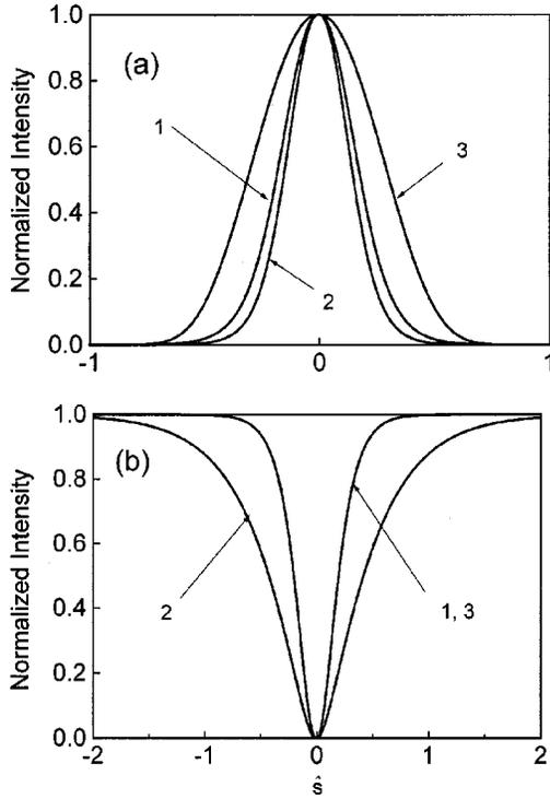
FIG. 4. Bright-dark separate screening soliton pairs in a biased series SBN crystal circuit. (a) Bright soliton profiles in the crystal  $P$ . (b) Dark soliton profiles in the crystal  $\hat{P}$ .
