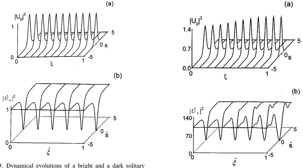
FIG. 9. Dynamical evolutions of a bright and a dark solitary states  $U_0$  and  $\hat{U}_0$  in a biased series SBN crystal circuit. (a) Bright soliton  $U_0$  in the crystal  $P$  and (b) Dark soliton  $\hat{U}_0$  in the crystal  $\hat{P}$ .
