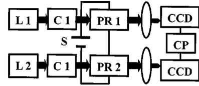
FIG. 2. An envisaged experiment arrangement.  $L1$  and  $L2$  are the lasers,  $C1$  and  $C2$  are the collimators,  $S$  is the voltage source,  $PR1$  and  $PR2$  are the PR crystals, and  $CP$  is a computer.
