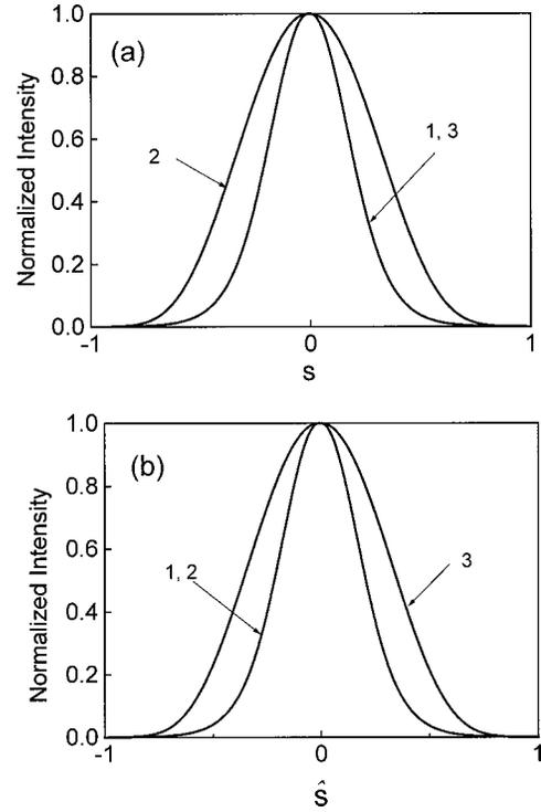
FIG. 5. Bright-bright separate screening soliton pairs in a biased series SBN crystal circuit. (a) Bright soliton profiles in the crystal  $P$ . (b) Bright soliton profiles in the crystal  $\hat{P}$ .
