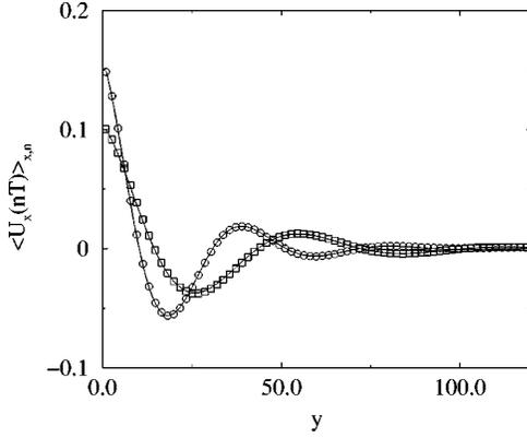
FIG. 3. Plots of the  $x$  component of the average velocity  $\langle U_x(y, t_n) \rangle_{x,n}$  measured at the times  $t_n = nT$ ,  $n = 1, \dots$ , vs the distance from the driving wall  $y$  for  $\nu = 0.042$  and  $\mu = 0.3$ . Simulation results for  $T = 2000$ ,  $\tau = 920$  and  $T = 4000$ ,  $\tau = 1840$  are shown by circles and squares, respectively. Solid lines correspond to theoretical results in the form  $\langle U_x \rangle = A \exp[-\text{Im}(k)y] \cos[\text{Re}(k)y]$ .
