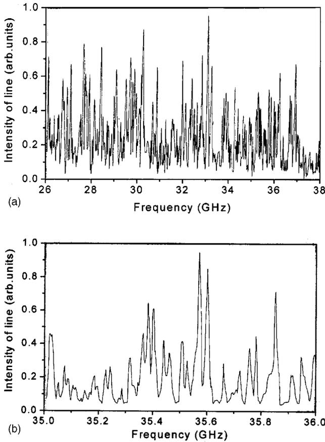
FIG. 2. (a) Total character of the QCR chaotic spectrum in all measured frequency bands 26–38 GHz. (b) The QCR chaotic spectrum in the narrow frequency range 35–36 GHz (one of realizations).
