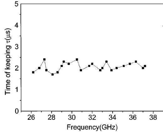
FIG. 7. Frequency dependence of keeping time of a microwave impulse in the QCR.
