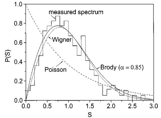
FIG. 3. Nearest-neighbor frequency spacing distribution. The histogram corresponds to the experimental data and the solid line shows the best fit with the Brody distribution. The short dotted line is the Wigner distribution and the dashed line is the Poisson distribution.
