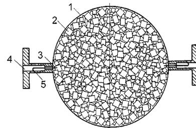
FIG. 1. Quasi-optical cavity resonator. (1) Metal cavity; (2) sapphire particles; (3) antenna; (4) wave guide; (5) loop coupler.
