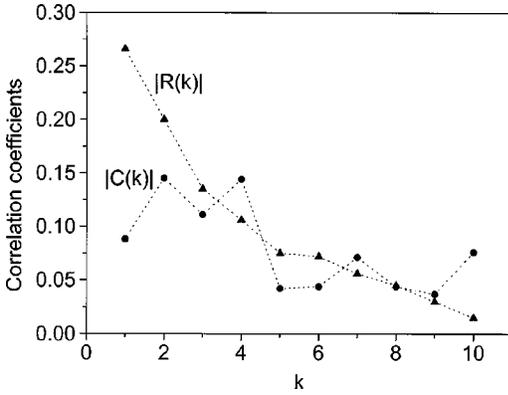
FIG. 4. Correlation properties of the quasioptical resonator spectrum. Nearest-neighbor frequency spacing correlations  $C(k)$ . The correlation of resonance line intensity on frequency  $R(k)$ . The scale on the X axis is as follows:  $\Delta k=1$  corresponds to  $\Delta f = 34.87\text{MHz}$ .
