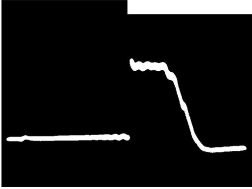
FIG. 6. Oscilloscope of a microwave impulse retained in a quasi-optical resonator. The sweep duration is  $10 \mu s$ .
