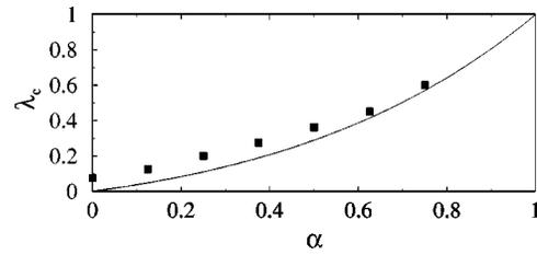
FIG. 3. The dependence of the epidemic threshold  $\lambda_c$  on  $\alpha$  as predicted by our calculations (continuous line) based on the continuum approach, and by the numerical simulations based on the SIS model (boxes). The small deviation between the numerical results and the analytical prediction is due to the uncertainty in determining the precise value of the threshold in Monte Carlo simulations.
