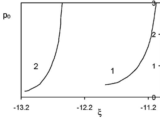
FIG. 2. Dependence of dimensionless electron initial momentum  $p_0$  on the trapping point near the first accelerating maximum. 1,  $a_0=2$ ; 2,  $a_0=3$ .
