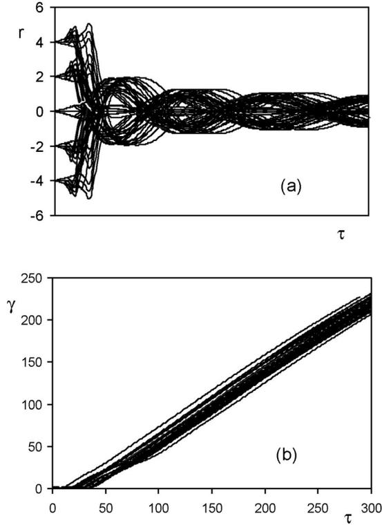
FIG. 12. Trapping, compression, and acceleration of an electron bunch in the wakefield presented in Fig. 7. Initial parameters of the bunch are:  $0 \leq \xi_0 \leq 5$ ,  $r_0 \leq 4$ ,  $0.6 \leq p_{z0} \leq 0.8$ ,  $-0.02 \leq p_{r0} \leq 0.02$ . The normalized radial positions (a) and relativistic factor (b) of electrons.
