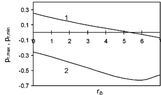
FIG. 11. Maximum (curve 1) and minimum (curve 2) dimensionless initial radial momenta of trapped electrons depending on the normalized initial radial position,  $p_{z0}=0.8$ ,  $\xi_0=0$ .
