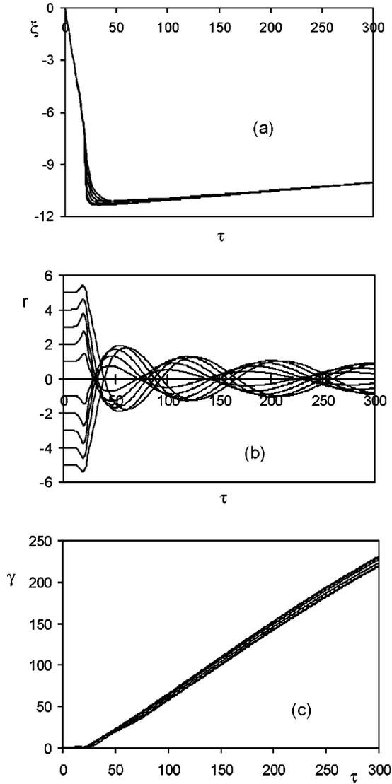
FIG. 9. Trapping and acceleration of electrons with zero initial momenta in the wakefield given in Fig. 7,  $p_{z0}=0.8$ ,  $\xi_0=0$ . Longitudinal (a) and radial (b) positions and relativistic factor (c) of electrons. The coordinates and time are normalized.
