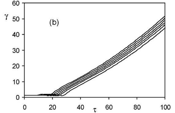
FIG. 4. Trapping, compression, and acceleration of the initially monoenergetic electron bunch in the wakefield presented in Fig. 1,  $p_0=0.5$ ,  $1 \leq \xi_0 \leq 6$ . Evolution of the coordinate (a) and the relativistic factor (b) of electrons. The coordinate and time are normalized.
