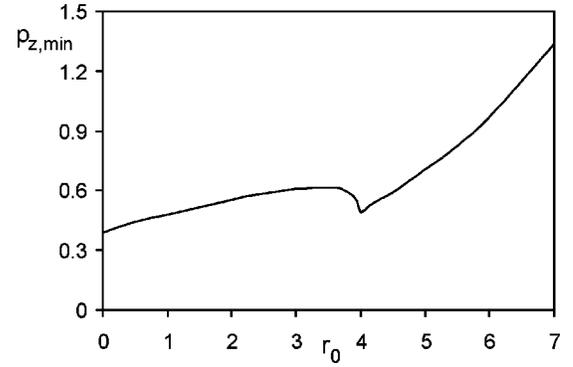
FIG. 10. The characteristic dependence of the minimum trapping threshold on the initial radial position of the electron,  $p_{r0}=0$ ,  $\xi_0=0$ . Both variables are dimensionless.
