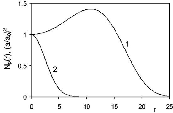
FIG. 6. The radial profiles of dimensionless unperturbed electron density in the plasma channel (curve 1) and the normalized laser-pulse intensity (curve 2),  $r_{ch} = \sigma_r = 5$ ,  $b = 0.01$ .
