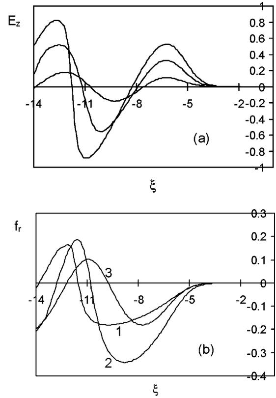
FIG. 7. The two-dimensional nonlinear laser wakefield excited in the plasma channel with the radial density profile shown in Fig. 6,  $a_0 = 2$ ,  $\sigma_z = 2$ ,  $\sigma_r = 5$ . (a) The longitudinal electric field for  $r_0 = 0, 3$ , and  $5$  in the order of magnitude reduction. (b) The focusing field  $f_r = \beta_g H_\theta - E_r$ . 1,  $r = 1$ ; 2,  $r = 3$ ; 3,  $r = 5$ . All variables are normalized.
