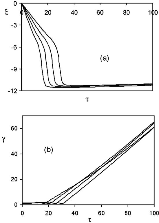
FIG. 5. Behavior of electrons with initial position  $\xi_0=0$  and with initial momenta  $p_0=0.5, 0.8, 1,$  and  $1.2$  in the wakefield shown in Fig. 1. Electrons with smaller initial momenta are trapped earlier. (a) The normalized coordinate and (b) relativistic factor of electrons.
