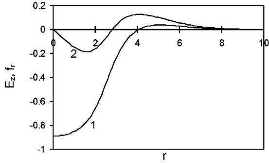
FIG. 8. The radial behavior of the wakefield shown in Fig. 7, at  $\xi = -10.9$ . 1, dimensionless longitudinal electric field  $E_z(\xi = -10.9, r)$ ; 2, the normalized focusing force  $f_r(\xi = -10.9, r)$ .
