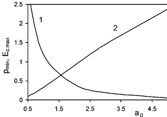
FIG. 3. The minimum dimensionless momentum of the trapped electrons  $p_{\min}$  (curve 1) and the normalized wake wave amplitude  $E_{z,\max}$  (curve 2) in dependence on peak amplitude of the laser pulse  $a_0$ .
