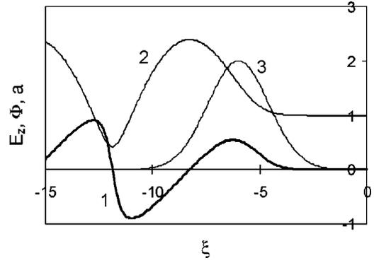
FIG. 1. The one-dimensional nonlinear wakefield excited by the linearly polarized laser pulse with peak normalized amplitude  $a_0 = 2$ ,  $\sigma_z = 2$ ,  $\gamma = 10$ . 1, the longitudinal electric field  $E_z(\xi)$ ; 2, the potential of the wakefield  $\Phi(\xi)$ ; 3, the amplitude of the laser pulse  $a(\xi)$ . All variables are normalized (see the text).
