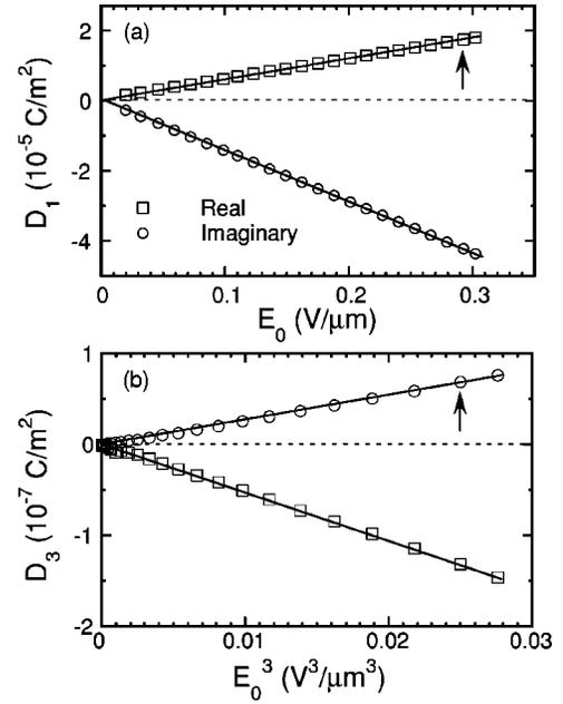
FIG. 3. Dependences of the real and imaginary parts of (a)  $D_1$  and (b)  $D_3$  on  $E_0^n$ , measured simultaneously at 1 kHz at  $102.10^\circ\text{C}$  just below the Sm-A–Sm- $C_\alpha^*$  phase transition point. The solid lines are the best fitting results of  $D_n = \varepsilon_n E_0^n$ .
