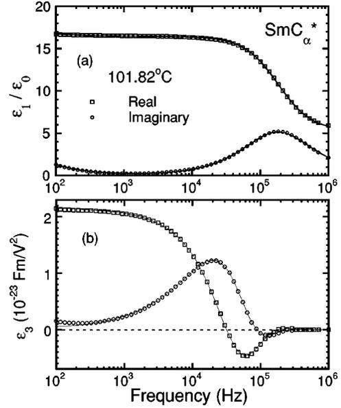
FIG. 7. Typical frequency dispersions of (a)  $\varepsilon_1(\omega)$  and (b)  $\varepsilon_3(\omega, \omega, \omega)$  obtained at 101.82 °C in the Sm- $C_\alpha^*$  phase. The solid lines represent the best fit results with Eq. (18) and Eq. (22) for the linear and third-order nonlinear dielectric dispersions, respectively.
