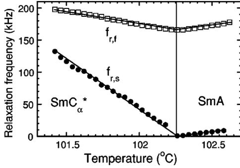
FIG. 8. Temperature dependences of the relaxation frequencies obtained from the linear and the third-order nonlinear dielectric spectroscopy.  $f_{r,f}$  and  $f_{r,s}$  are the relaxation frequencies of the ferroelectric mode and the soft mode, respectively.
