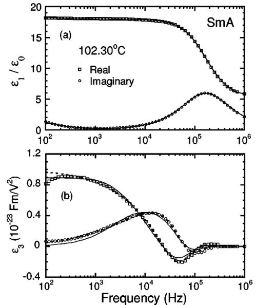
FIG. 6. Typical frequency dispersions of (a)  $\varepsilon_1(\omega)$  and (b)  $\varepsilon_3(\omega, \omega, \omega)$  obtained in the Sm-A phase (102.30 °C). The solid lines represent the best fit results with Eq. (18) and Eq. (21) for the linear and the third-order nonlinear dielectric dispersions, respectively. In (b), the broken line is the best fit with the distribution parameter  $\beta$ .
