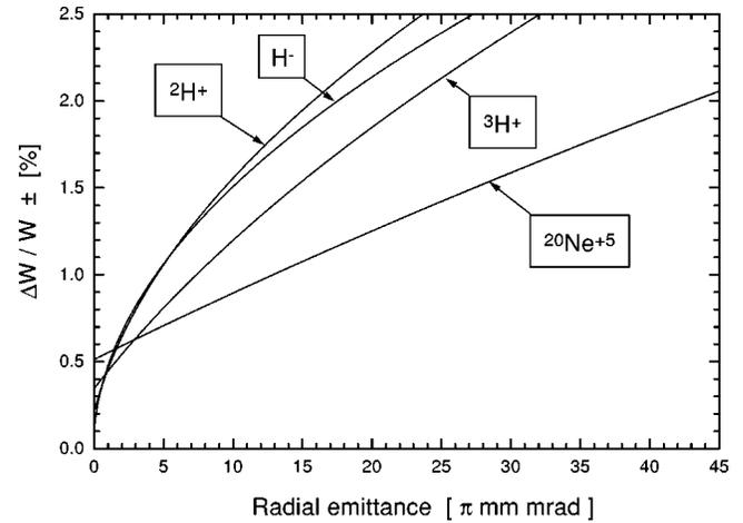
FIG. 6. Energy spread of the beam on a stripping foil vs its radial emittance for four types of ions.
