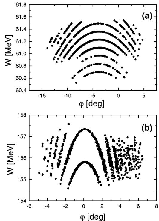
FIG. 4. Distribution of particle energy on the SF for (a)  $H^-$  and (b)  $^{20}\text{Ne}^{5+}$  ions vs their rf phase.
