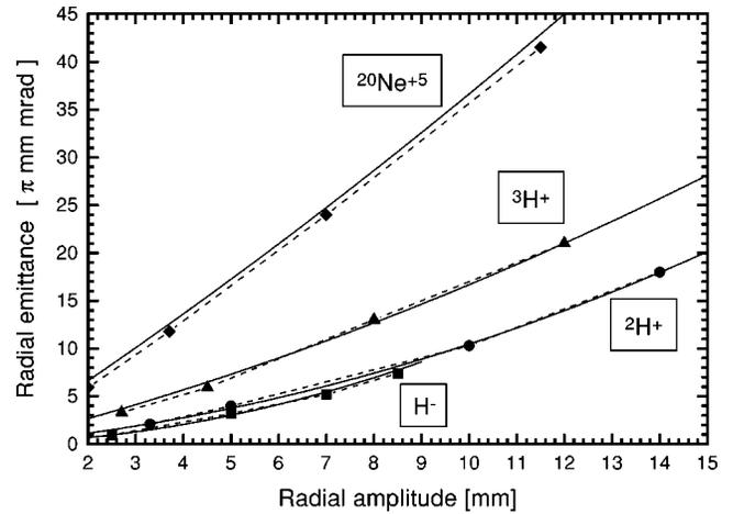
FIG. 3. Radial emittances on a stripping foil vs amplitude of the radial oscillations inside the circulating beam. Solid lines, analytical estimates; points and dashed lines, numerical calculations for four types of ions.
