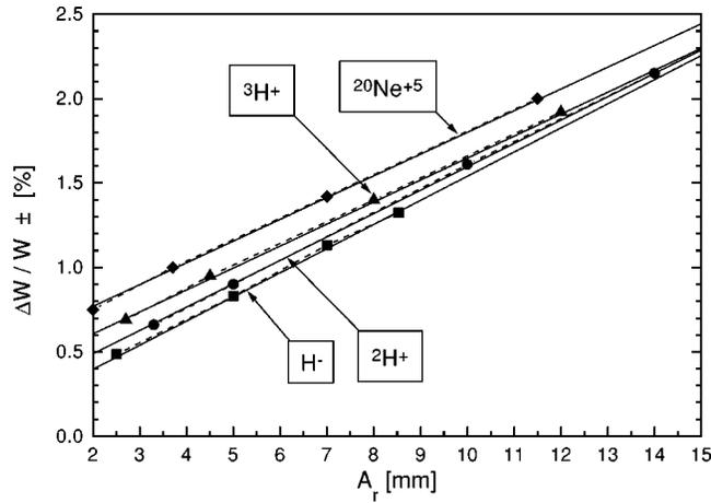
FIG. 5. Relative energy spread for four types of ions as a function of radial amplitude: analytical estimates (solid lines) and results of numerical calculations (points and dashed lines).
