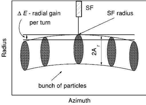
FIG. 1. Schematic view of the bunch of particles in the vicinity of the stripping foil.
