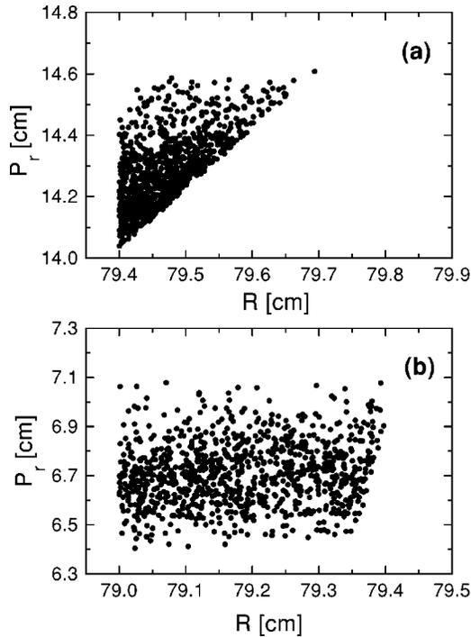
FIG. 2. Radial emittances on the stripping foil for  $H^-$  (a) and  $^{20}\text{Ne}^{5+}$  (b) ions.
