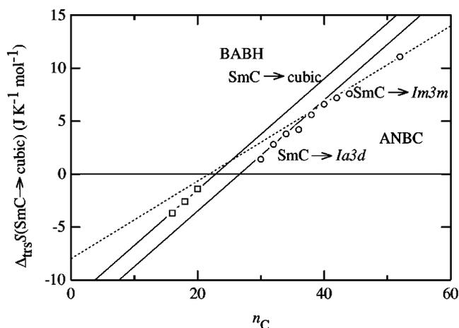
FIG. 6. Entropy of Sm-C → cubic transition in ANBC(*n*) and BABH(*n*). The  $n_C$  stands for the number of paraffinic carbon atoms attached to the constituting “molecule.” Here the “molecule” means a dimer in the case of ANBC and mole is applied to monomer for BABH and dimer for ANBC. The relation  $n_C = 2n$  holds for both because of its doubled structure of BABH molecule and of dimerization of ANBC molecules.
