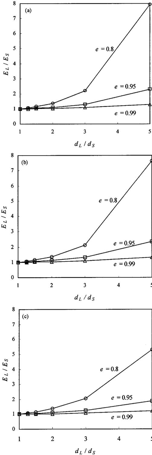
FIG. 6. Dependency of granular energy ratio ( $E_L/E_S$ ) on diameter ratio and restitution coefficient for  $\nu=0.3$  and (a)  $\nu_L/\nu_S=1.0$ , (b)  $\nu_L/\nu_S=0.5$ , and (c)  $\nu_L/\nu_S=4.0$ .
