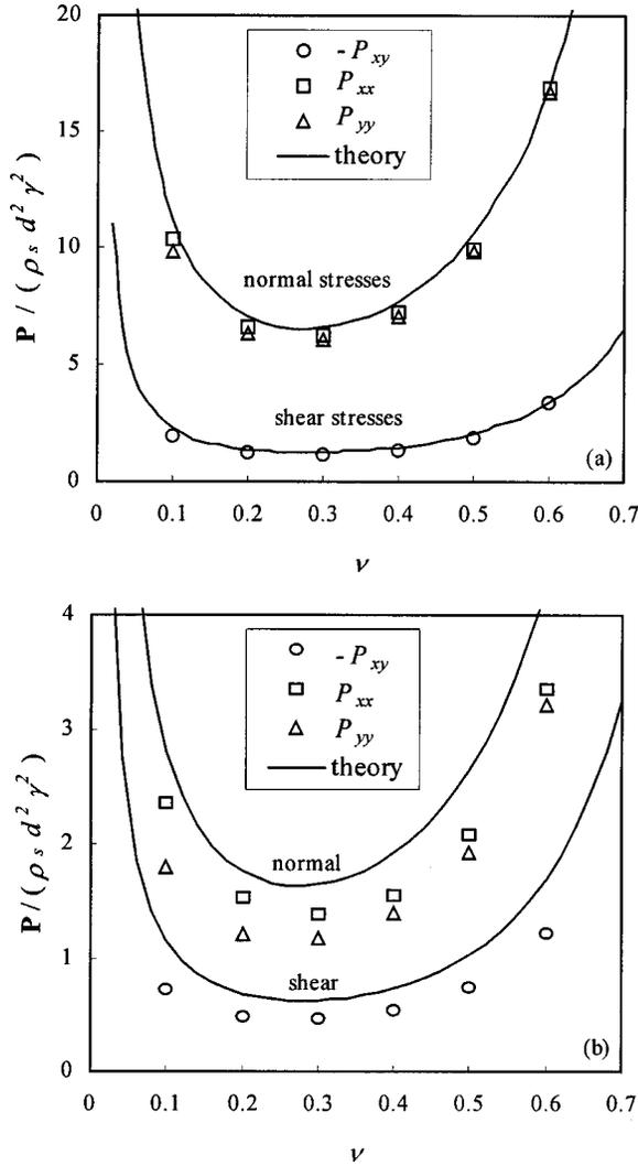
FIG. 2. Stresses in monodisperse systems with kinetic-theory predictions of Jenkins and Richman [16] for (a)  $e=0.95$  and (b)  $e=0.8$ .
