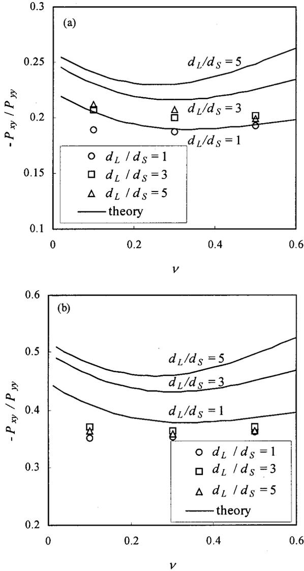
FIG. 8. Dynamic friction coefficients for binary systems with kinetic-theory predictions of Willits and Arnason [9] for  $\nu_L/\nu_S = 1.0$  and (a)  $e = 0.95$  and (b)  $e = 0.80$ .
