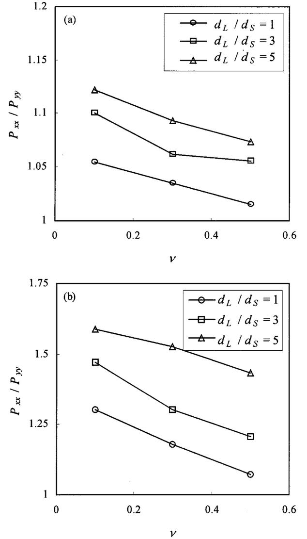
FIG. 9. Normal stress ratios for binary systems with  $\nu_L/\nu_S = 1.0$  and (a)  $e = 0.95$  and (b)  $e = 0.8$ .
