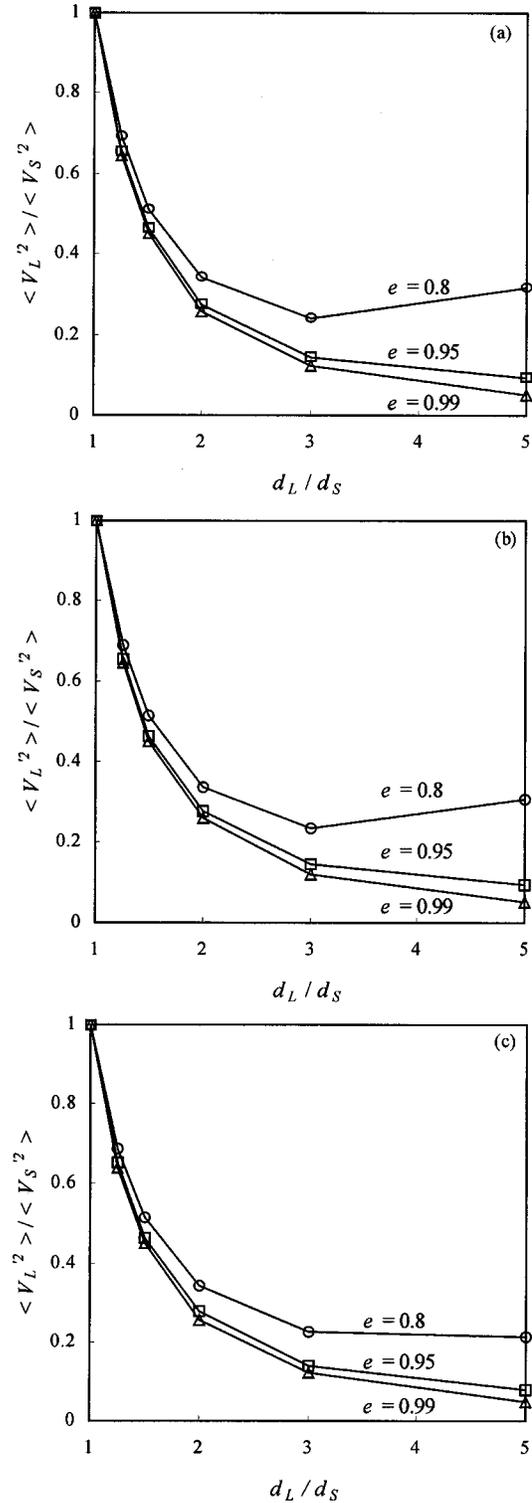
FIG. 7. Dependency of square of fluctuating velocity ratio ( $\langle V_L'^2 \rangle / \langle V_S'^2 \rangle$ ) on diameter ratio and restitution coefficient for  $\nu=0.3$  and (a)  $\nu_L/\nu_S=1.0$ , (b)  $\nu_L/\nu_S=0.5$ , and (c)  $\nu_L/\nu_S=4.0$ .
