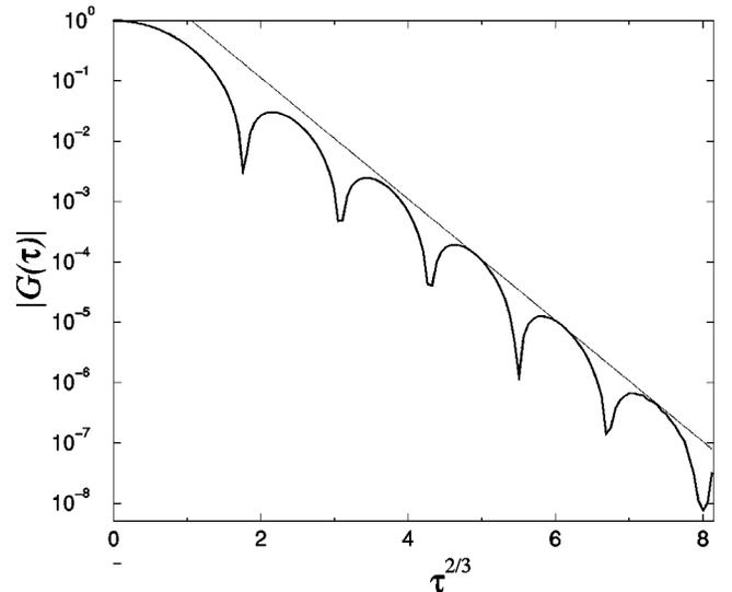
FIG. 2. Oscillation and stretched exponential behavior in the response function  $G(\tau)$ . The straight line indicates a line of slope  $-1$  as predicted by Eq. (7).
