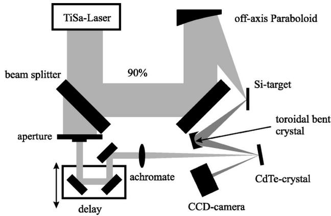
FIG. 1. The Ti:sapphire laser system delivers pulses of about 80 fs with a pulse energy of 200 mJ. 90% of the energy is focused onto a silicon target by an off-axis paraboloid, producing a short burst of Si  $K\alpha$  line emission. A fraction of the 10% transmitted laser energy is used to induce changes in the lattice properties of the CdTe crystal layer. The changes are probed by the silicon  $K\alpha$  pulse and detected by an x-ray CCD camera.
