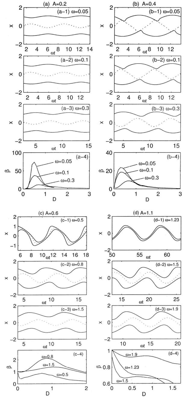
FIG. 7. The deterministic trajectories (phase portraits cut along one generator of the cylinder and developed to a plane; solid line: SLC, dashed line: ULC) and the curves of  $\beta$  vs  $D$  for the cases of  $A=0.2$  (a),  $A=0.4$  (b),  $A=0.6$  (c),  $A=1.1$  (d), and various values of  $\omega$ .
