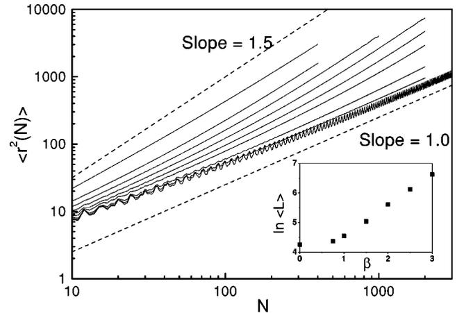
FIG. 2. Log-log plot of the mean square end-to-end distance as a function of  $N$  for  $\beta=0, 1.0, 1.5, 2.0, 2.5, 3.0, 4.0, 5.0$ , and 300, from top to bottom. Inset: Logarithm of the mean trapping length,  $\ln \langle L \rangle$  as a function of  $\beta$ .
