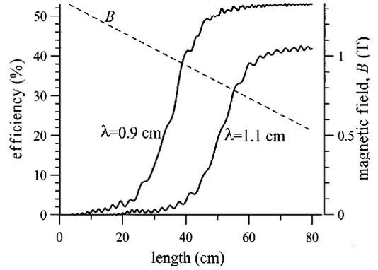
FIG. 6. Electronic efficiency versus the longitudinal coordinate at various wavelengths of the input signal (solid curves), and distribution of the magnetic field (dashed curve). The spread in oscillatory velocity is  $\epsilon=20\%$ , the magnetic field profile is  $\tilde{b}_{\max}=1.5$  and  $\tilde{b}_{\min}=0.7$ .
