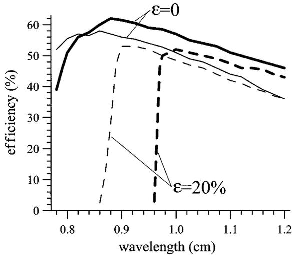
FIG. 7. Electronic efficiency versus the wavelength of the input signal. The magnetic field profile is  $\bar{b}_{\max}=1.5$  and  $\bar{b}_{\min}=0.7$ . The phase velocity at the center of the band ( $\lambda_c=1$  cm) is  $\beta_\phi^c=1.15$  (thin curves) and  $\beta_\phi^c=1.30$  (bold curves). The spread in oscillatory velocity is  $\epsilon=0$  (solid curves) and  $\epsilon=20\%$  (dashed curves).
