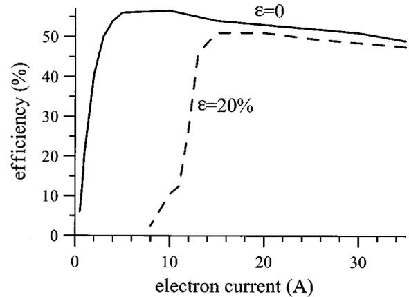
FIG. 8. Electronic efficiency versus the electron current in the cases of the spread in oscillatory velocity  $\epsilon=0$  (solid curve) and  $\epsilon=20\%$  (dashed curve). The magnetic field profile is  $\bar{b}_{\max}=1.5$  and  $\bar{b}_{\min}=0.7$ ; the phase velocity is  $\beta_\phi=1.30$ .
