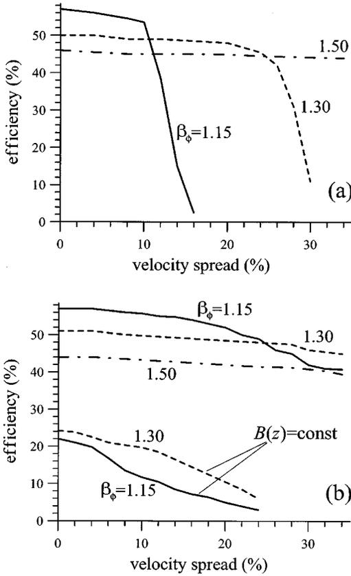
FIG. 5. CARM amplifier in the regime of nonresonant trapping. Electronic efficiency versus the spread in oscillatory velocity at various values of the phase velocity of the rf wave,  $\beta_\phi$ , and at different profiles of magnetic field: (a)  $\tilde{b}_{\max}=1.3$  and  $\tilde{b}_{\min}=0.7$ , (b)  $\tilde{b}_{\max}=1.5$  and  $\tilde{b}_{\min}=0.7$ . In (b), the two lower curves correspond to the regime of inertial electron bunching with uniform magnetic field.
