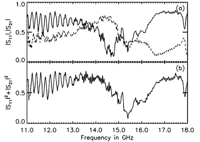
FIG. 2. (a) Reflection amplitude  $|S_{11}|$  (solid line) and transmission amplitude  $|S_{12}|$  (dashed line) of the ferrite used in the experiment, for an applied magnetic field  $B=0.475$  T. The oscillations observed for frequencies below 14 GHz are an artifact of the measurement. (b) Plot of  $|S_{11}|^2+|S_{12}|^2$ . The deep minimum at 15.4 GHz, reflecting strong absorption, is caused by the ferromagnetic resonance.
