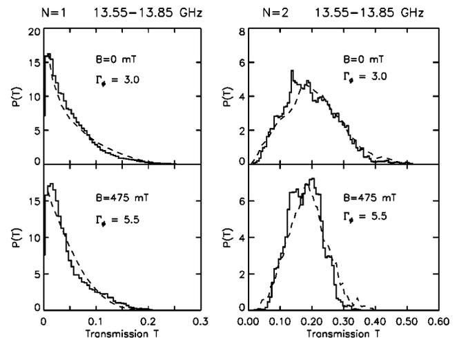
FIG. 4. Comparison of the experimental transmission intensity distributions with the theoretical calculations with absorbing channels (for details see text).
