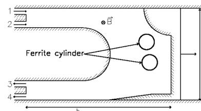
FIG. 1. Sketch of the used microwave resonator (in scale).
