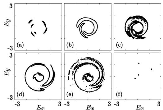
FIG. 7. Breakup of a torus and sudden disappearance of chaos at a saddle-node bifurcation of periodic orbits (intermittent transition); (a) and (b)  $\omega=0.43$ ,  $K=0.1139, 0.1145$ , and from (c) to (f)  $\omega=0.42$ ,  $K=0.12, 0.145, 0.166, 0.167$ .
