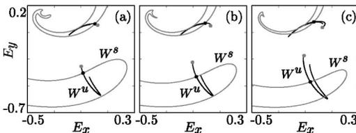
FIG. 15. Formation of homoclinic tangle of the black periodic orbit (originally on the chaotic attractor), demonstrating that Fig. 13 indeed shows a boundary crisis;  $K=0.2885$  and from (a) to (c)  $\omega$  takes the values 0.255, 0.26, and 0.275.
