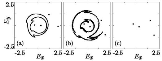
FIG. 10. A sudden destruction of the chaotic attractor (created in the breakup of a torus, and coexisting with the gray attracting periodic orbit) in a boundary crisis; from (a) to (c)  $\omega=0.46$  and  $K$  takes the values 0.115, 0.129, and 0.13.
