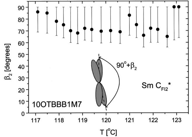
FIG. 10. Temperature dependence of the calculated distortion angle  $\beta_2$  in the smectic- $C_{F12}^*$  phase of 10OTBBB1M7.
