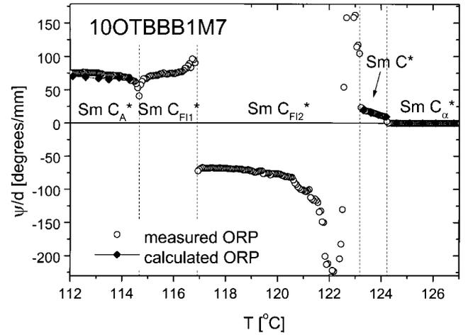
FIG. 6. Temperature dependence of the measured ORP (○) in 10OTBBB1M7 [18] together with the calculated ORP (◆). The calculations were made within Yeh's formalism.
