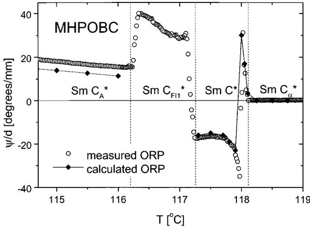
FIG. 5. Temperature dependence of the measured ORP (○) in MHPOBC [4] together with the calculated ORP (◆). The calculations were made within Yeh's formalism.
