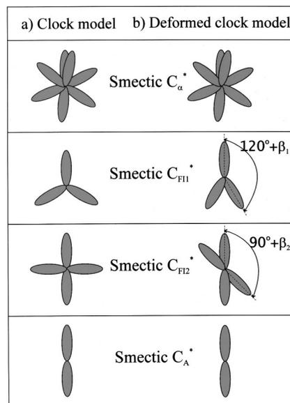
FIG. 1. (a) The set of tilted phases of polar smectics, as reproduced within the “clock” model of Čepič and Zekš. (b) The proposed structures, based on experimental evidence from ellipsometry and ORP measurements.
