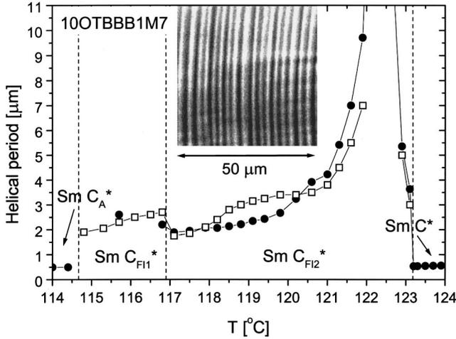
FIG. 8. Temperature dependence of the helical period in the smectic- $C_{F11}^*$  and smectic- $C_{F12}^*$  phases of 10OTBBB1M7, measured directly by the observation of disclination lines (open squares) and determined indirectly from relaxation rates of the phase mode (filled circles). The inset shows a picture of disclination lines under polarizing microscope in the smectic- $C_{F12}^*$  phase at the temperature of 118.5°C.
