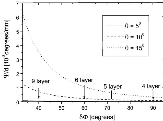
FIG. 3. Optical rotatory power of smectic- $C^*$  phase as a function of the phase difference between the directions of directors in neighboring smectic layers  $\delta\Phi$ , calculated for different values of the tilt angle. The wavelength of light is 632.8 nm and the eigenvalues of the dielectric tensor are  $\epsilon_1 = 2.28$  and  $\epsilon_3 = 2.89$ , ORP was calculated within Yeh's  $4 \times 4$  matrix formalism.
