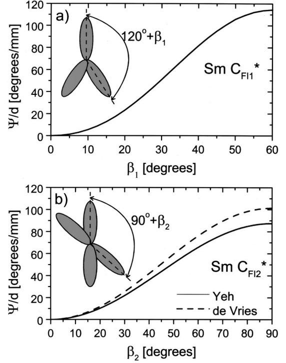
FIG. 4. Optical rotatory power of (a) the three-layer smectic- $C^*_{F11}$ , (b) the four-layer smectic- $C^*_{F12}$  ferroelectric phase as a function of the angle of distortion of a unit cell, indicated in the inset. Yeh's formalism was used with  $\lambda = 632.8$  nm,  $\epsilon_1 = 2.28$ ,  $\epsilon_3 = 2.89$ ,  $p = 3$   $\mu\text{m}$ , and  $\theta = 17^\circ$ . The dashed line in Fig. 4(b) is de Vries's calculation according to Eqs. (11) and (12) with the same set of parameters.
