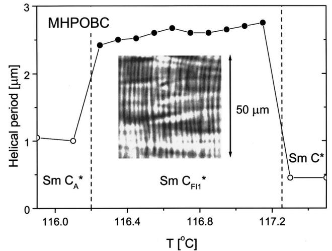
FIG. 7. Temperature dependence of the helical period in the smectic- $C_{FI1}^*$  phase of MHPOBC, measured by the observation of disclination lines (filled circles). The values in the smectic- $C^*$  and smectic- $C_A^*$  phase are from Ref. [17] (open circles). The inset shows a picture of disclination lines of the smectic- $C_{FI1}^*$  phase under polarizing microscope at the temperature of  $116.5^\circ\text{C}$ .
