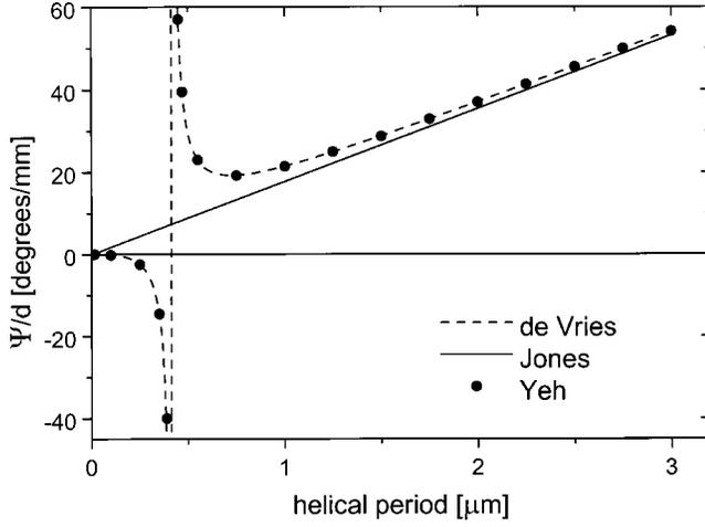
FIG. 2. Comparison of optical rotatory power of ferroelectric smectic- $C^*$  phase, calculated from de Vries's analytical solutions of the wave equation, Yeh's  $4 \times 4$  matrix approach, and Jones matrix formalism as a function of helical period. The tilt angle is  $16.2^\circ$ , whereas the eigenvalues of the dielectric tensor are  $\epsilon_1 = 2.28$  and  $\epsilon_3 = 2.89$ , the wavelength of light is 632.8 nm.
