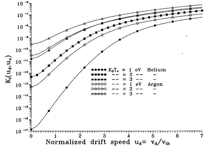
FIG. 1. Impact ionization reaction rate for helium (solid symbols) and argon (open symbols) at different drift speeds and several electron temperatures for drifting electron populations.
