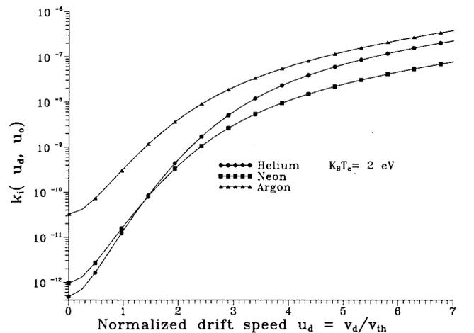
FIG. 2. Comparison of impact ionization reaction rates for different atomic gases at a fixed kinetic temperature of drifting electron population.
