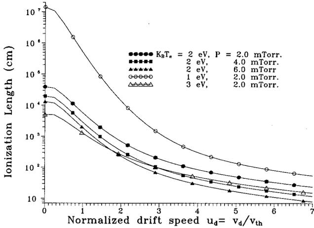
FIG. 3. Characteristic ionization length for typical electron temperatures and neutral pressures in Argon for different normalized drift speeds.
