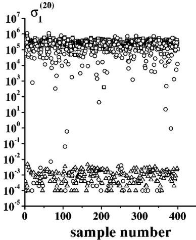
FIG. 4. The first moment of the distribution of exchange energies after 20 RG iterations, for each single sample, at  $p=0.892$  and three different temperatures. (a) Along the Nishimori line (squares); (b)  $k_B T/J=0.5$  (circles); (c) Zero temperature (triangles). For a better visualization, the samples with  $\sigma_1^{(20)} < 10^{-5}$  were not represented.
