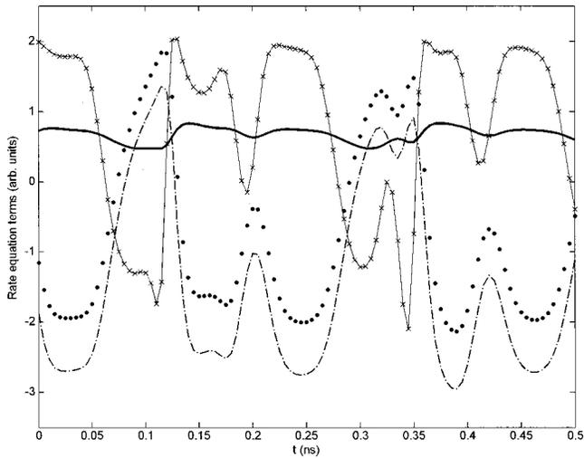
FIG. 2. Conventional synchronization. Contributions to the evolution of  $aE_T(t-\tau_c)$  given by Eq. (7) and  $E_R(t)$  given by Eq. (4): first term of the right-hand side of Eq. (7) (dots); feedback term in Eq. (7) (crosses); first term of the right-hand side of Eq. (4) (dash-dot); feedback term in Eq. (4) (thin solid line); external injection term in (4) (thick solid line).
