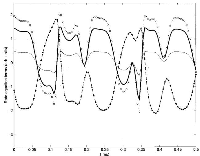
FIG. 4. Anticipating synchronization. Contributions to the evolution of  $E_T(t - \tau_c + \tau)$  given by Eq. (9) and  $E_R(t)$  given by Eq. (4): first term of the right-hand side of Eq. (9) (dots); feedback term in Eq. (9) ( $\dots \times \dots$ ); first term of the right-hand side of Eq. (4) (dash-dot); feedback term in Eq. (4) (thin solid line); external injection term in (4) (thick solid line). The origin of time is not the same as in Fig. 2.
