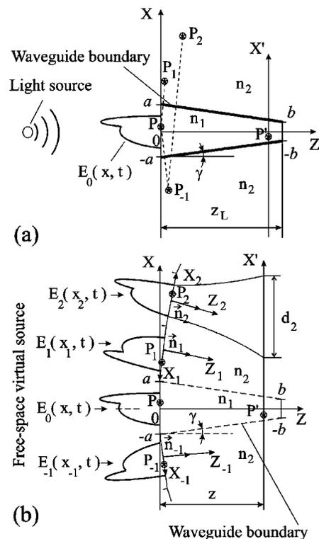
FIG. 1. (a) Propagation of the wave through the tapered optical waveguide. (b) Schematic diagram of the free-space virtual source.
