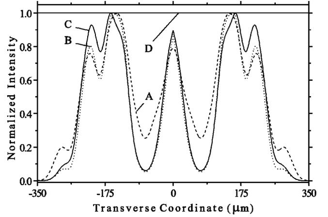
FIG. 6. Normalized intensity distributions of the partially coherent field at the guide exit computed using Eqs. (10)–(14). The parameters of the light at the guide entrance: A,  $|\mu| = 1$ ; B,  $|\mu| = 0.85$ ; C,  $|\mu| = 0.75$ ; and D,  $|\mu| = 0$ .
