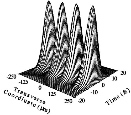
FIG. 5. The normalized intensity distributions of the pulse having  $E_0(x) = \text{TE}_3(x)$  calculated using Eqs. (1)–(7) for the different distances  $z=0, 5, 10 \text{ cm}$  from the virtual source. The respective distributions obtained using the conventional theory of waveguides are shown for comparison.
