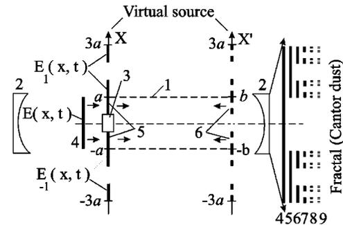
FIG. 7. Formation of the laser fractal (Cantor dust) in the waveguide resonator: 1, guide boundary; 2, mirrors, and 3, obstacle. The triadic Cantor discontinuum (line fractal): 4,  $C_0$ ; 5,  $C_1$ ; 6,  $C_2$ ; 7,  $C_3$ ; 8,  $C_4$ ; and 9,  $C_5$ .
