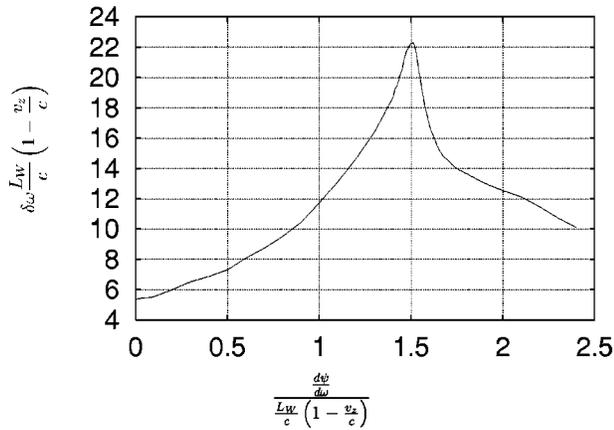
FIG. 6. Dependence of the FEL gain width on the dispersion parameter  $d\psi/d\omega$ . It is seen that gain exists for all FEL frequencies at which strong interaction with the ponderomotive potential occurs. The same type of dependence appears for drift regions shown in Figs. 4 and 5. The parameter space is different, but in both cases there is a parameter region where broadband gain exists (normalized by  $T$  as in Figs. 2 and 4).
