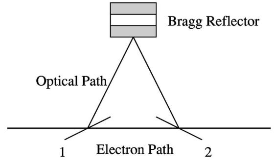
FIG. 5. Scheme of the drift region with a Bragg reflector for a broadband FEL.
