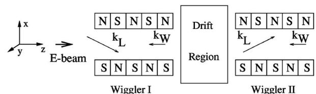
FIG. 1. Two coupled wigglers separated by a drift region.
