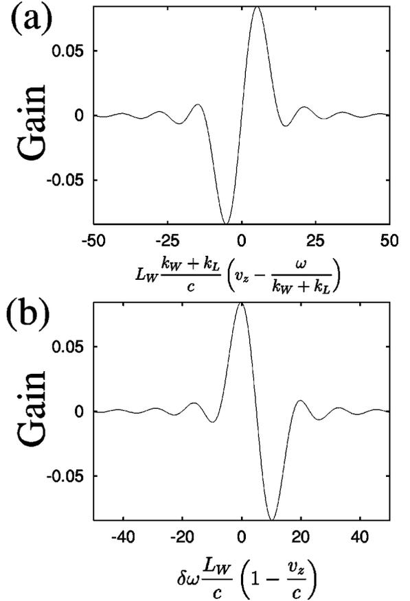
FIG. 2. Gain (arbitrary units) dependence on detuning  $\Omega$  as a function of (a)  $\delta v_z = v_z - \omega / (k_W + k_L)$  and (b) laser frequency variation  $\delta\omega$ , for the ordinary free electron laser. The frequency variation is normalized by the interaction time in the wiggler  $T = L_W / c(1 - v_z / c)$ .
