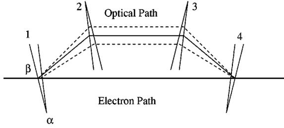
FIG. 4. Scheme of the drift region with prisms for a broadband FEL (or optical phased klystron).
