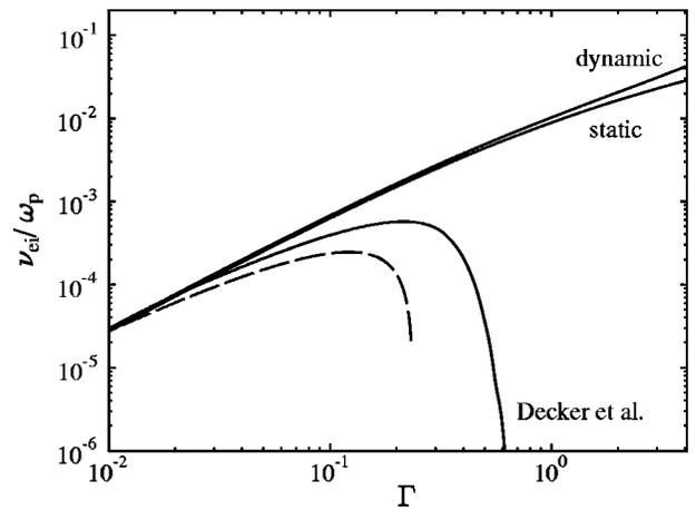
FIG. 5. Electron-ion collision frequency as a function of the coupling parameter  $\Gamma$  for a hydrogen plasma in a laser field ( $Z = 1; v_0/v_{th} = 10; n_e = 10^{22} \text{ cm}^{-3}; \omega/\omega_p = 5$ ). Comparison is given with the theory of Decker *et al.* and with the asymptotic formula (45) of Silin (dashed line).
