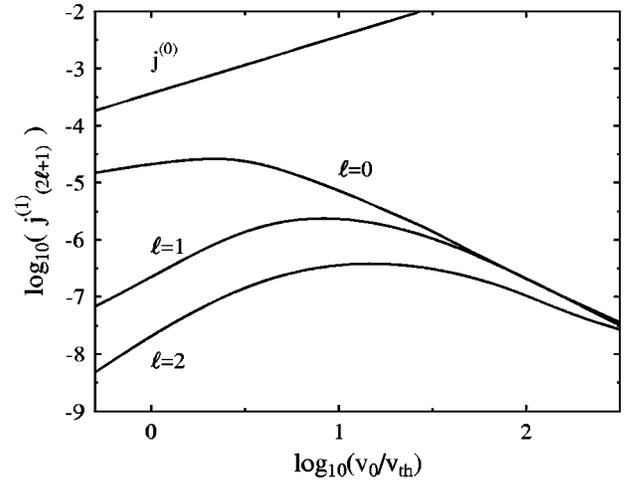
FIG. 9. Amplitudes  $2\sqrt{(\text{Re}j_m)^2 + (\text{Im}j_m)^2}$  of the  $m=(2\ell+1)$ th harmonics of the current vs field strength denoted by  $v_0/v_{th}$ . The parameters are  $n_e = 4 \times 10^{21} \text{ cm}^{-3}$  and  $T = 1.2 \times 10^5 \text{ K}$ .
