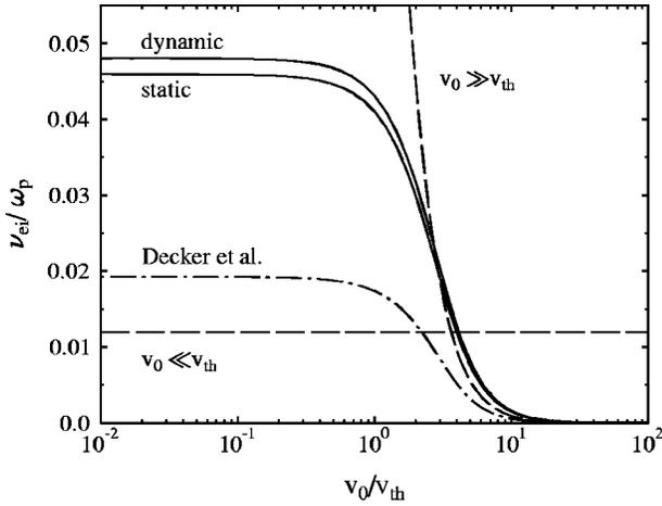
FIG. 2. Electron-ion collision frequency vs quiver velocity for the same parameters as in Fig. 1.
