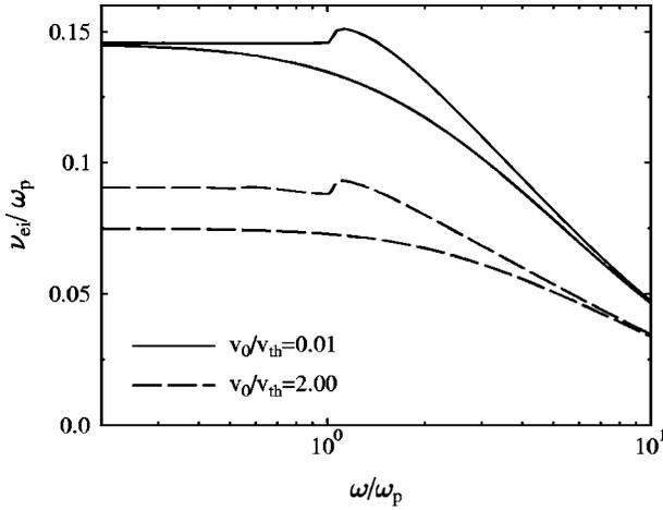
FIG. 8. Electron-ion collision frequency as a function of the laser frequency for a hydrogen plasma ( $n_e = 10^{21} \text{ cm}^{-3}$ ;  $T = 10^5 \text{ K}$ ) for two different field strengths. The upper curve of each pair corresponds to the full dynamical screening, the lower one to the static screening approximation.
