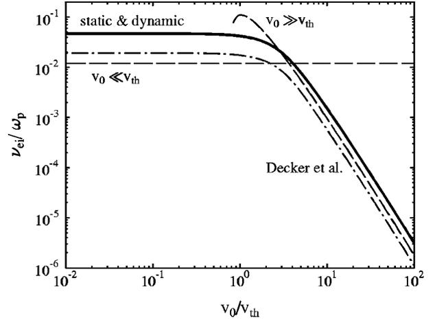
FIG. 1. Electron-ion collision frequency as a function of the quiver velocity  $v_0 = eE/\omega m_e$  for a hydrogen plasma in a laser field ( $Z=1; n_e = 10^{22} \text{ cm}^{-3}; T = 3 \cdot 10^5 \text{ K}; \omega/\omega_p = 5$ ). For comparison, results of Decker *et al.* (dash-dotted line) and of the asymptotic formulas (44) and (45) of Silin (dashed line) are given.
