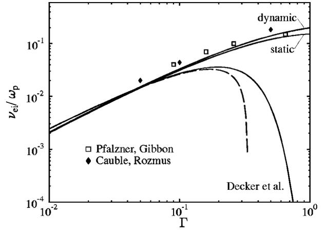
FIG. 4. Electron-ion collision frequency as a function of the coupling parameter  $\Gamma$  for a hydrogen plasma in a laser field ( $Z = 1; v_0/v_{th} = 0.2; n_e = 10^{22} \text{ cm}^{-3}; \omega/\omega_p = 3$ ). Comparison is given with the theory of Decker *et al.* and with the asymptotic formula (44) of Silin (dashed line).
