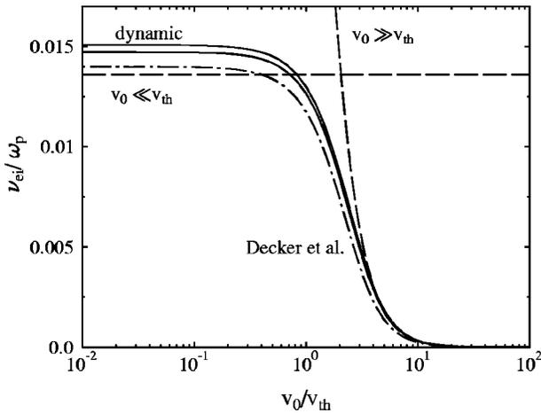
FIG. 3. Electron-ion collision frequency as a function of the quiver velocity  $v_0 = eE/\omega m_e$  for a hydrogen plasma in a laser field ( $Z = 1; n_e = 10^{22} \text{ cm}^{-3}; T = 10^6 \text{ K}; \omega/\omega_p = 5$ ). For comparison, results of Decker *et al.* (dash-dotted line) and of the asymptotic formulas (44) and (45) of Silin (dashed line) are given.
