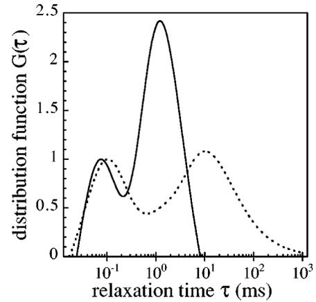
FIG. 7. Relaxation time distribution functions corresponding to aging times  $t_w=0$  (full line) and  $t_w=400$  mins (dashed line) for a 2.5% wt suspension. The corresponding autocorrelation functions are taken under a scattering angle  $\theta=90^\circ$ . In order to be able to compare the functions, the peak intensities for the small-scale Brownian motion were normalized to unity.
