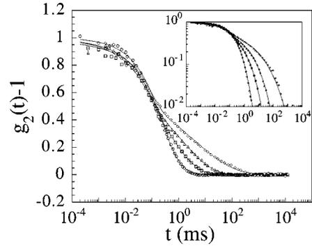
FIG. 2. Autocorrelation functions of the scattered intensity by a 2.5% wt suspension and corresponding fits for aging times  $t_w = 0, 200, 400, 600 \text{ min}$  (from left to right) at a scattering angle  $\theta = 90^\circ$ . The autocorrelation functions and their corresponding fits are also represented on a log-log plot in inset.
