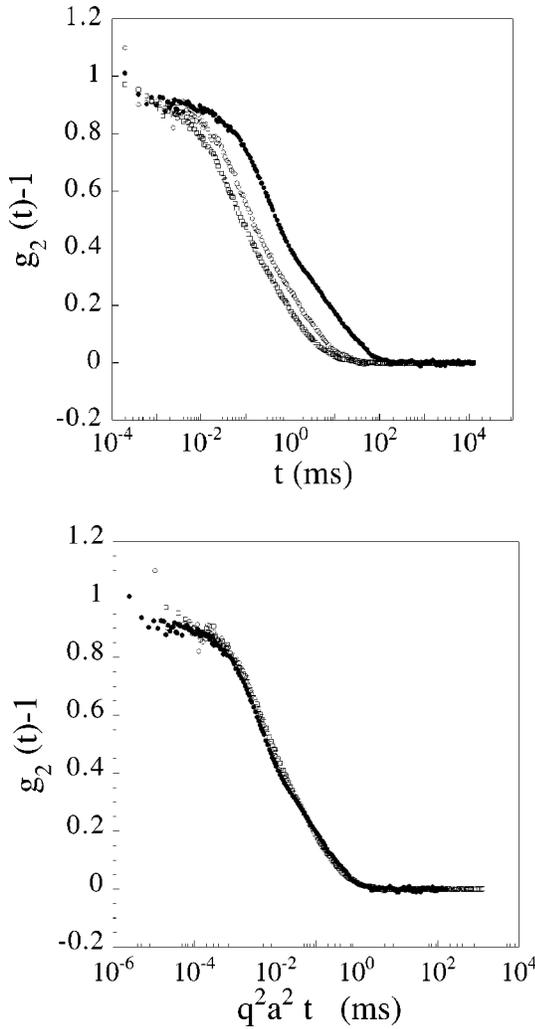
FIG. 6. Scaling of the autocorrelation functions taken under different scattering angles  $\theta=40^\circ$  (open squares),  $\theta=90^\circ$  (open circles), and  $\theta=150^\circ$  (filled circles), for an aging time  $t_w=300$  min (2.5% wt).  $a$  is the radius of the particles [8]
