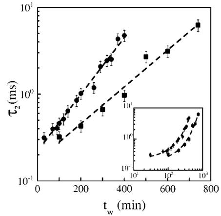
FIG. 4. Characteristic time  $\tau_2$  of the slow relaxation as a function of the aging time for 2.5% wt (squares) and 2.8% wt (circles) Laponite suspensions from autocorrelation functions taken under a scattering angle  $\theta = 90^\circ$ .  $\tau_2(t_w)$  is also represented on a log-log plot in the inset.
