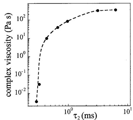
FIG. 8. Complex viscosity as a function of  $\tau_2$  for a 2.5% wt Laponite suspension for a pulsation  $\omega=1$  s $^{-1}$ .
