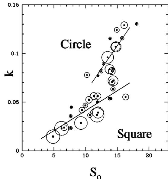
FIG. 4. Analysis of the axial segregation time dependence in the square and circular mixers. The curves from Fourier analysis are fitted to an exponential curve of the form  $s = S_0(1 - e^{-kt})$ , where  $k$  is in  $(\text{rot})^{-1}$ . The diameter of the circles represents the quality of the fitting given by the value of the correlation coefficient; small circles represent good fit. The range of correlation coefficients for these data is from 0.91 to 0.99.
