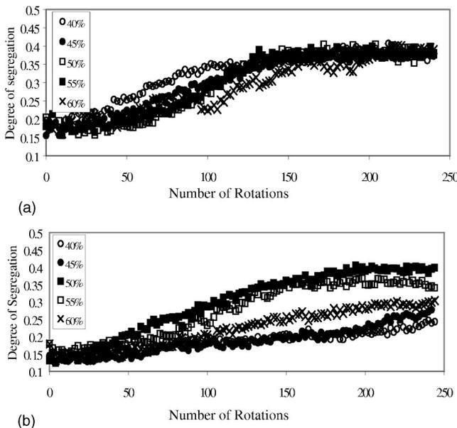
FIG. 3. Results from segregation measurements using the standard deviation about the mean concentration (a measure of the intensity of segregation) for the circle (a) and the square (b). The data are normalized so that a value of 0.5 would mean complete segregation of the two particles. Plots indicate that the segregation dynamics are virtually independent of filling fraction for the circular tumbler and sensitive to fill level for the square mixer.
