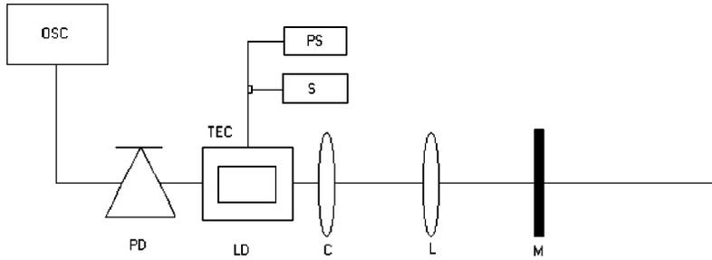
FIG. 1. Experimental setup: LD: laser diode; PD: photodiode; OSC: oscilloscope; C: collimator; L: lens; M: mirror; TEC: thermoelectric cooler; PS: power source; S: wave form generator.
