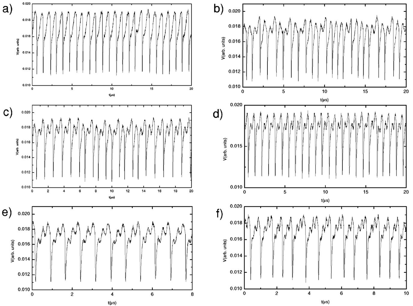
FIG. 2. Time series corresponding to every one of the experimentally observed behaviors. (a) 1:1 pattern. (b) Intermittencies between the 1:1 and the 1:2 patterns. (c) 2:3 pattern. (d) 1:2 pattern. (e) 1:3 pattern. (f) Intermittencies between the 1:3 and the 1:4 pattern.
