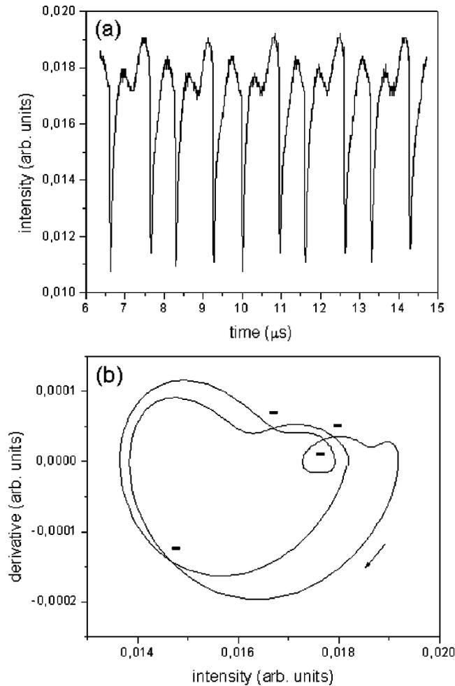
FIG. 6. (a) Experimental time series with the 2:3 pattern. (b) Embedding of the corresponding time series. The mathematical symbols display the orientation of the crossing. The topological numbers were computed in the  $(x, t)$  projection.
