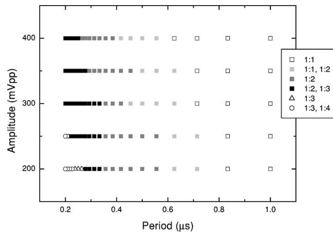
FIG. 3. The experimental map of the regions in which the different periodic patterns have been observed. The amplitude is in unit of millivolts peak to peak (mVpp).
