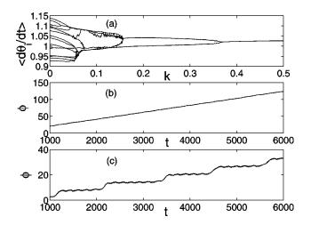
FIG. 1. For a system of 15 coupled Rössler chaotic oscillators: (a) the average frequencies vs the coupling parameter K, (b) linear growth of the phase difference between two clusters for  $K=0.005 < K_m = 0.024$ , and (c)  $2\pi$  phase jumps preceding the merger of the clusters for K=0.022.
