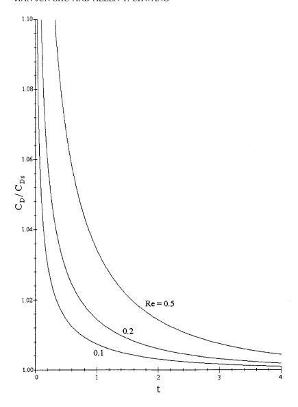
FIG. 1. Ratio of unsteady to steady drag coefficient for a sphere versus time for  $\Omega = 0$ .
