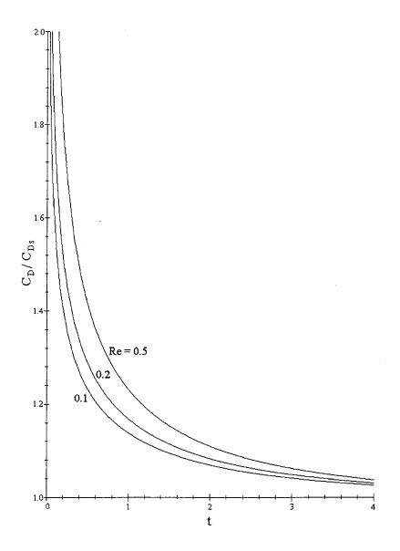
FIG. 2. Ratio of unsteady to steady drag coefficient for a circular cylinder versus time.
