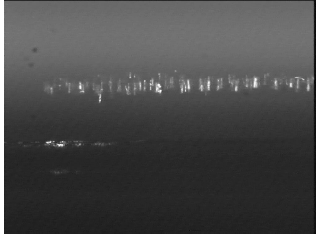
FIG. 2. As in Fig. 1 but as seen from the side. The background shows some variation of the plasma visible emission through a 633 nm filter. On the lower left we can see the reflection from the confining rig. The region of horizontal levitation is on the right; note two horizontal particles.
