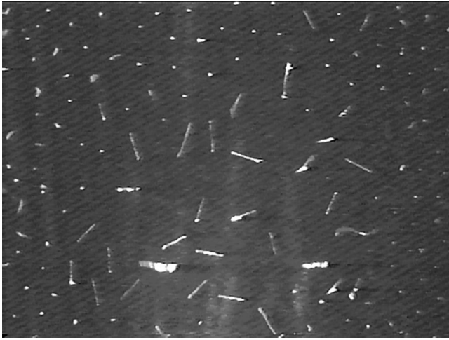
FIG. 1. The levitation of the 7.5 \mu\text{m} diameter rods in a krypton plasma at 52 Pa and 80 V rf as seen from the top. The dots are vertical rods.
