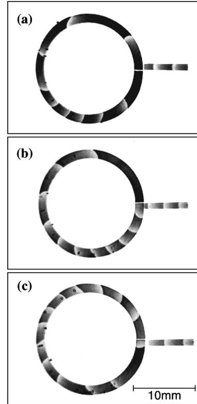
FIG. 4. Real-time memory in a real experiment (catalyst-doped BZ medium). (a) Successive input signals are introduced into the ring memory through the channel, and the pulses continue to rotate in the counterclockwise direction. (b) The input channel is shifted to a lower position, and input signals are then newly memorized as clockwise traveling waves. (c) Even after the input channel is disconnected, the memorized signals continue to rotate clockwise.
