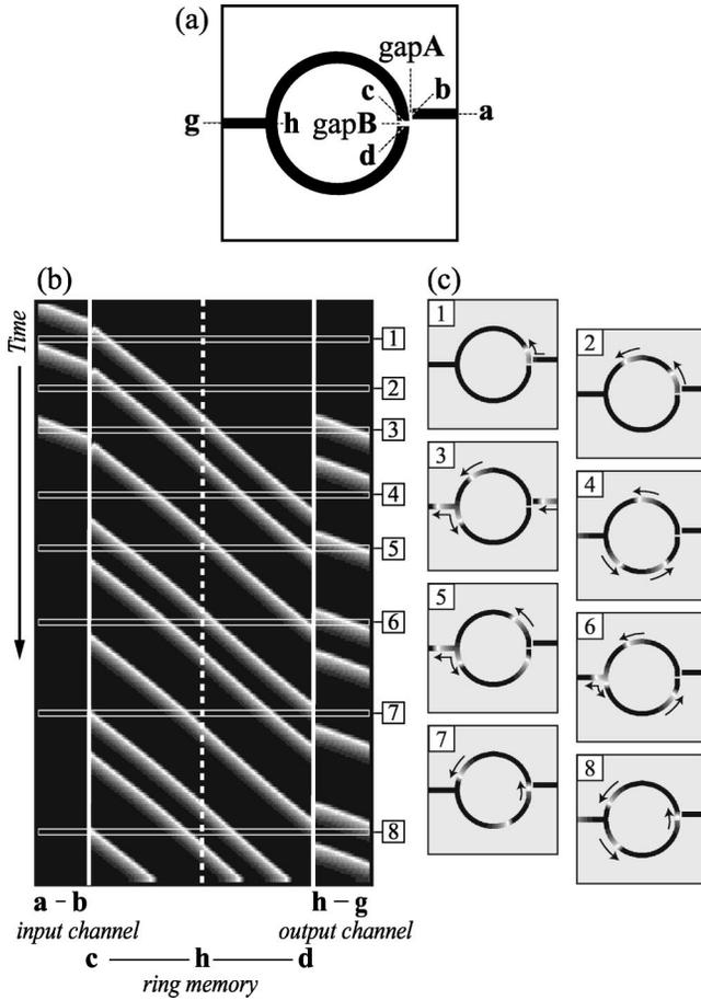
FIG. 3. (a) Geometry of the memory device equipped with an output channel  $h-g$ . (b) Space-time plot of traveling waves. Three successive input signals are introduced to the ring memory, and the three pulses are read out repeatedly through channel  $h-g$ . The broken line indicates the position of the output channel [ $h$  in (a)]. (c) Snapshot of the traveling waves.
