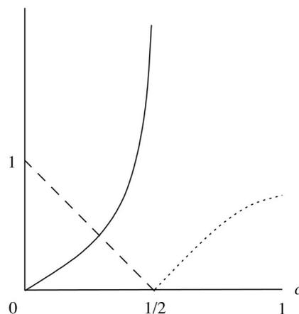
FIG. 1. Sketch of some critical quantities for gelation as a function of the crosslink concentration  $c$  for a mean-field distribution of crosslinks. The gelation transition occurs at  $c_{\text{crit}} = \frac{1}{2}$ . The plot displays the averaged static shear viscosity (solid line) according to Eq. (3.26), the effective diffusion constant (dashed line) according to Eq. (4.17) and the gel fraction (dotted line) according to Ref. [8].
