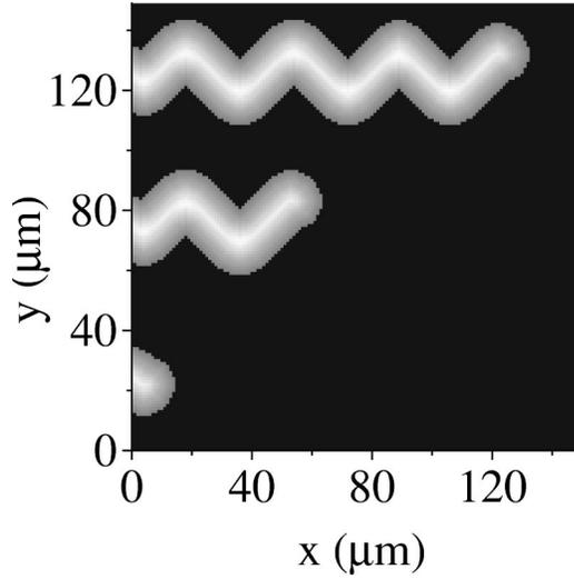
FIG. 2. A blister is represented at three different stages of its growth, the strain is  $\epsilon^* = 0.0085$ . On the gray scale, the sharp fold (the highest values of  $\zeta$ ) is represented with white color. The laminated part of the film is black colored. The selected directions of growth are selected by the square meshing.
