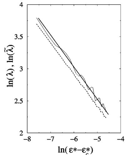
FIG. 4. Strain dependence of  $\lambda$  (solid line) and  $\tilde{\lambda}$  (dashed line). The straight line indicates  $\sim -\frac{1}{2}$  slope.  $\epsilon_c^* \approx 0.006$ .  $\lambda$  and  $\tilde{\lambda}$  are in  $\mu$ m, and they are averaged on ten periods of blister undulations.
