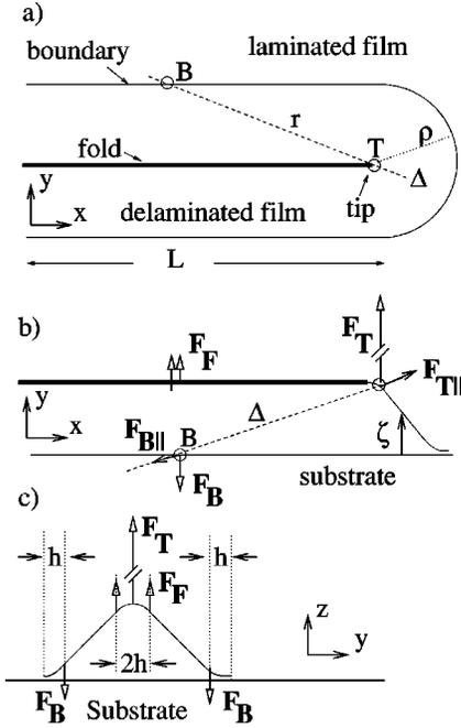
FIG. 1. Seed blister. (a) above view, (b) side view, and (c) front view. The bold line represents the fold obtained by Eq. (1). The slope  $k$  of the delaminated film and the ratio  $h/\rho$  are exaggerated for clarity.
