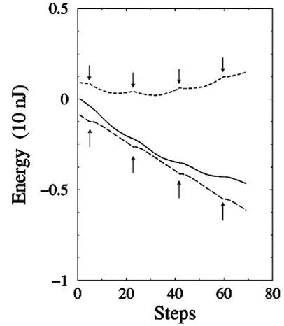
FIG. 3. Energy variation during the growth. Dotted line,  $E_{tens}$ ; dashed line,  $E_{delam}$ ; solid line,  $E_{el}$ . Arrows indicate changes of direction. The strain is  $\epsilon^* = 0.0085$ .
