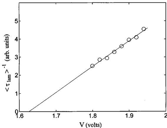
FIG. 3. Evolution of the inverse of the mean laminar duration as a function of the control parameter (bias of the source plasma). The critical value of the control parameter is close to 1.65. A linear law is recorded.
