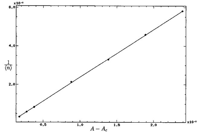
FIG. 6. Inverse of the mean duration of laminar phases as a function of the distance of the control parameter  $A$  to its critical value (model).
