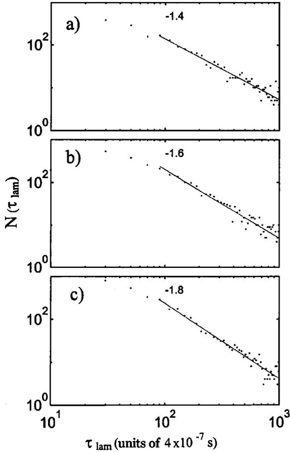
FIG. 2. Distribution of the duration of the laminar phases on a log-log plot for three different values of the control parameter (voltage between the plasma chambers). A power law of exponent  $-1.4$  is recorded at the threshold. This value decreases toward  $-2$  when the control parameter is increased.
