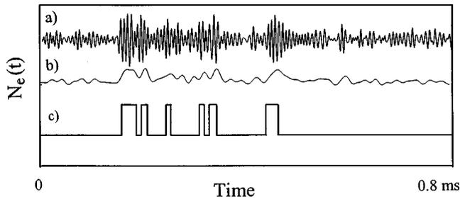
FIG. 1. Typical time series of the density fluctuations recorded on a plane probe in the target plasma 1 cm behind the grid, just at the onset of the instability. Bursts of high frequency waves can be clearly seen (a). The corresponding rectified and low pass filtered signal is displayed on trace (b). Binarization of the time series produces trace (c). The statistics of the laminar phase duration is investigated using this last signal.
