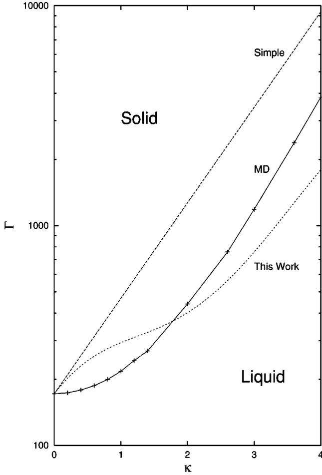
FIG. 3. Phase diagram of the Yukawa system in the  $\{\Gamma, \kappa\}$  plane. The liquid-solid phase boundary is shown as predicted by the simple estimate  $\Gamma = 171.8 \exp(\kappa)$  (top line), the solution of Eq. (18), and the simulation results of Hamaguchi *et al.* (line with circles). The results of this work are seen to give the phase boundary fairly well considering the simplicity of the theory.
