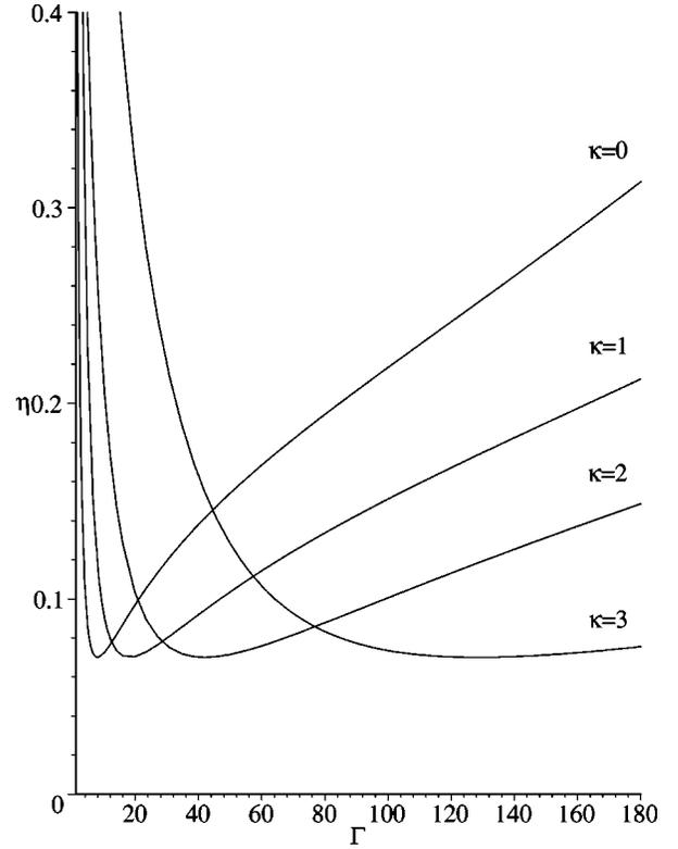
FIG. 4. The viscosity versus  $\Gamma$  for various values of  $\kappa$ . The  $\kappa=0$  case is the Wallenborn-Baus OCP result and the remaining curves are the corresponding Yukawa estimates based on Eq. (15).
