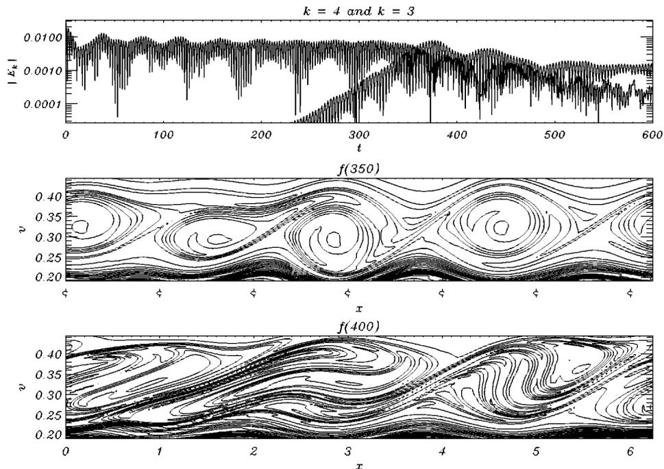
FIG. 6. Onset of the sideband instability ( $\epsilon=0.25$ ): (top) Semilogarithmic plot of  $|E_k|$  versus  $t$  for  $k=4$  and  $k=3$ ; (middle) contour plot of the EDF in the resonant region at  $t=350$ ; and (bottom) at  $t=400$ .
