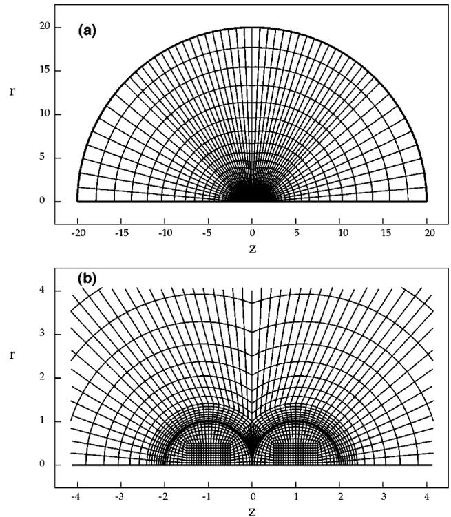
FIG. 2. Finite-element mesh for two touching spheres: (a) general view; (b) detail around touching spheres.
