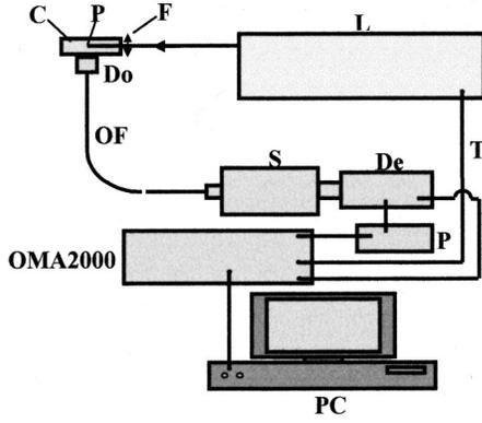
FIG. 1. *Experimental setup.* L=laser; F=focusing lens; P=plasma; C=cell; Do=imaging doublet; OF=optical fiber; S=spectrometer; De=intensified detector; T=electrical trigger; P=pulsar; OMA2000=optical multichannel analyzer; PC=personal computer.
