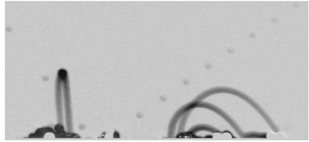
FIG. 9. An example of a collision showing ejectas taking off at a distance of about 10 grain diameters from the impact point.
