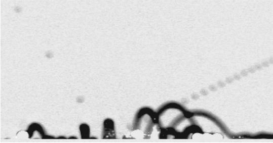
FIG. 2. Typical picture of a collision: the incident grain is coming from the left-hand side of the picture.
