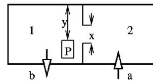
FIG. 1. Sketch of the twin microwave cavity. The antennas  $a$  and  $b$  are coupled to the generator and to the detector, respectively. The wall between the two cavities has an opening of width  $x$ , which couples them. The body  $P$  depicts a small block of plastics, which can be moved inside cavity 1 by an amount  $y$  from the wall.
