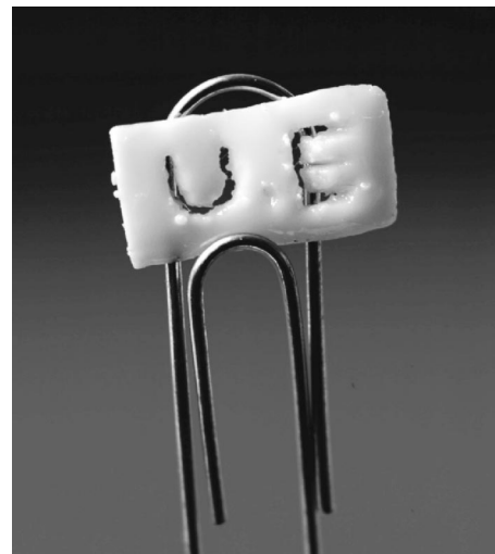
FIG. 1. A slice of the colloid–liquid-crystal composite, particle volume fraction \phi = 20\% . At room temperature it is sufficiently rigid to slice with a knife and engrave. It is shown resting on a paper clip to illustrate sample dimensions.
