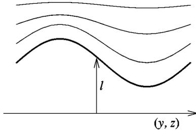
FIG. 1. Fluctuations  $l(y, z)$  of the SC/N interface (bold line) away from the  $(y, z)$  plane bend the lines of magnetic flux (thin lines), giving rise to an anisotropic  $|\mathbf{q}|$  contribution to the capillary wave energy [Eq. (5)]. For long wavelength fluctuations, this effect dominates the usual  $\mathbf{q}^2$  term that is generated by the surface tension.
